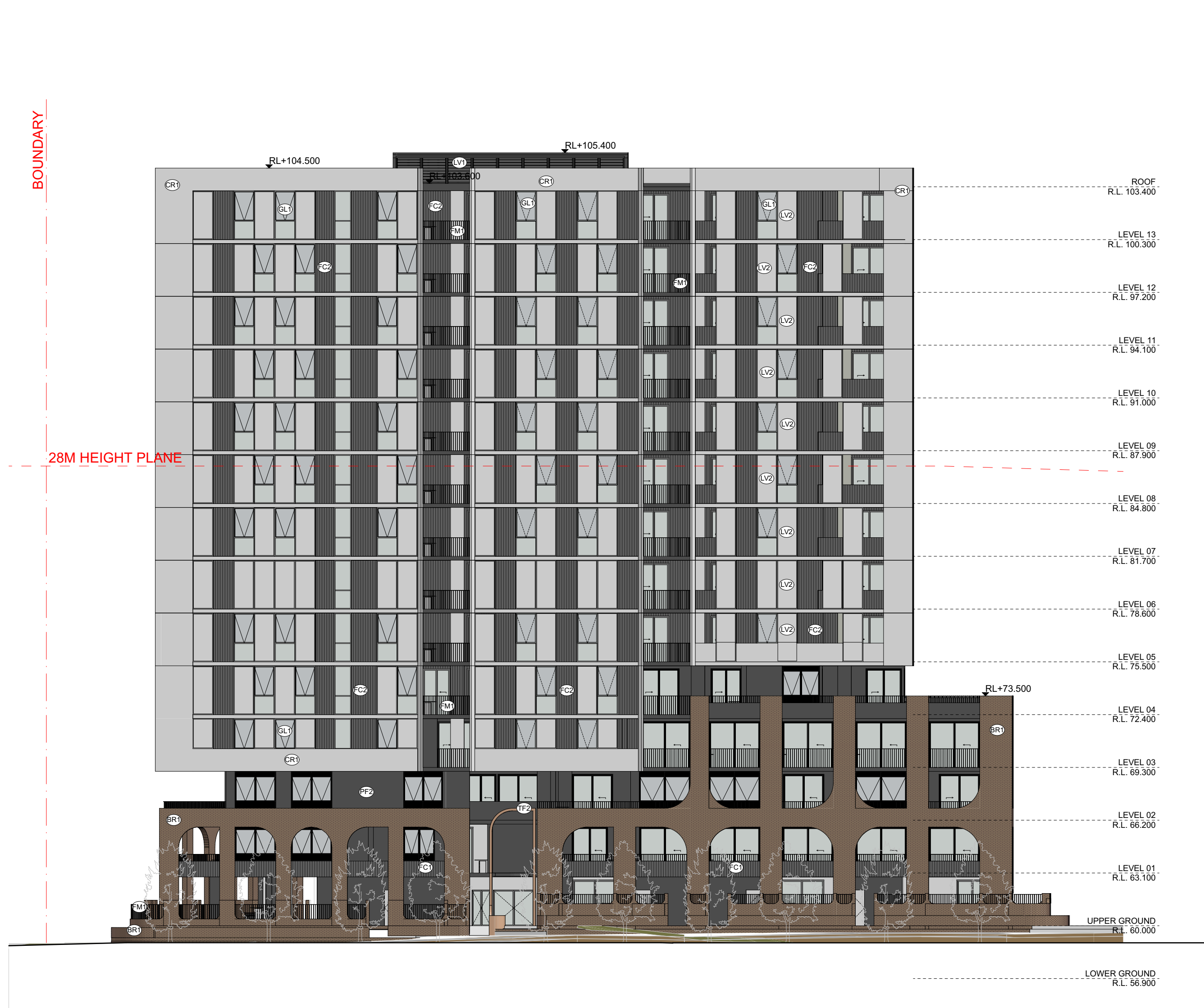
BW BLD. B WEST ELEVATION SCALE: 1:200@A1
