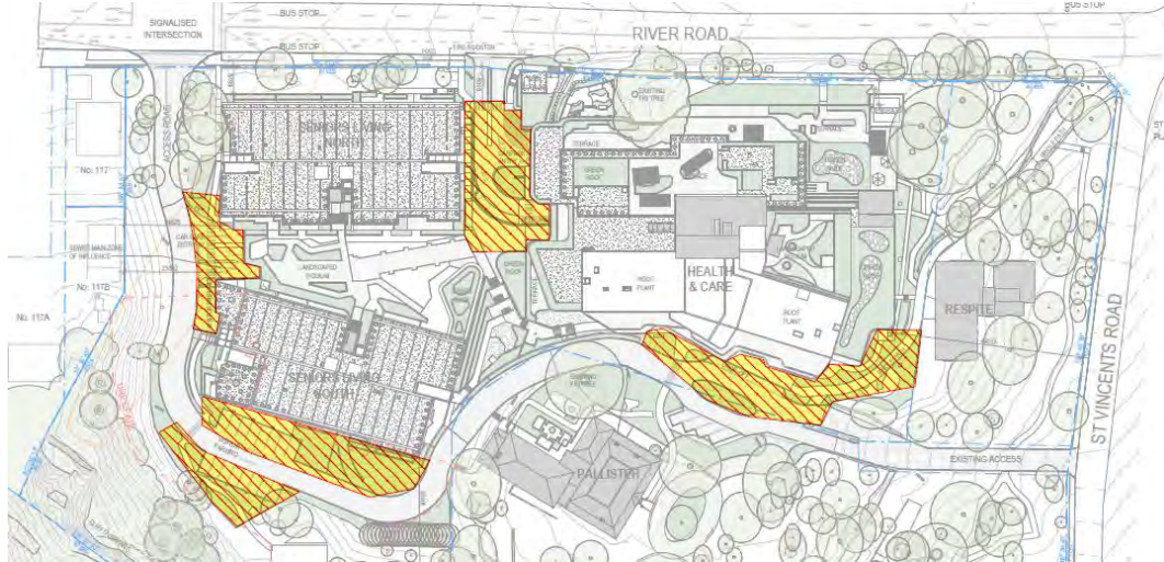
Figure 1: Proposed Materials Handling and Lay Down Areas
