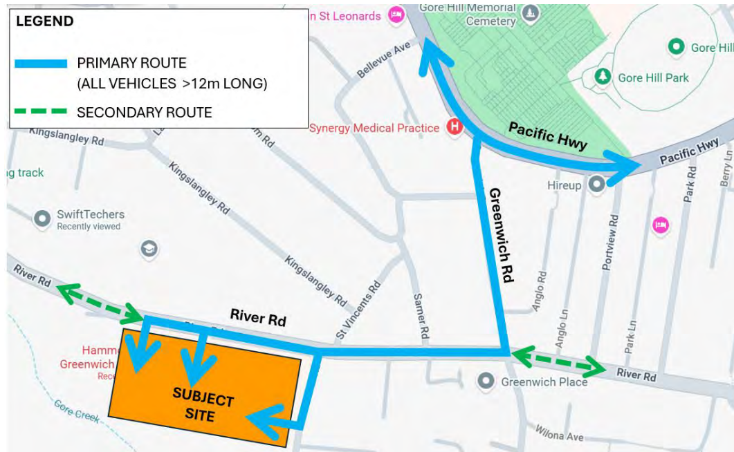
Figure 18: Primary Haulage and Secondary Access Routes
