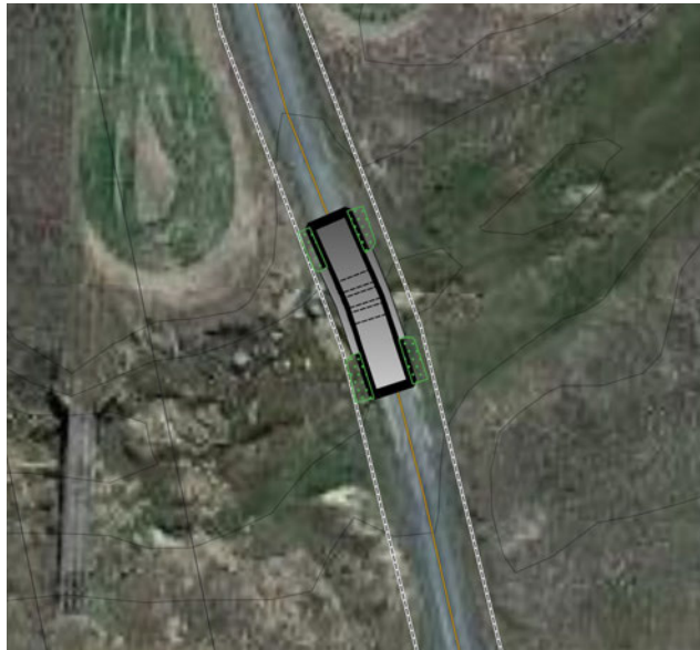
Figure 9-5. Proposed new crossing over Blind Creek. Concrete deck to be approximately 5m wide (Source: Stride Renewables).
