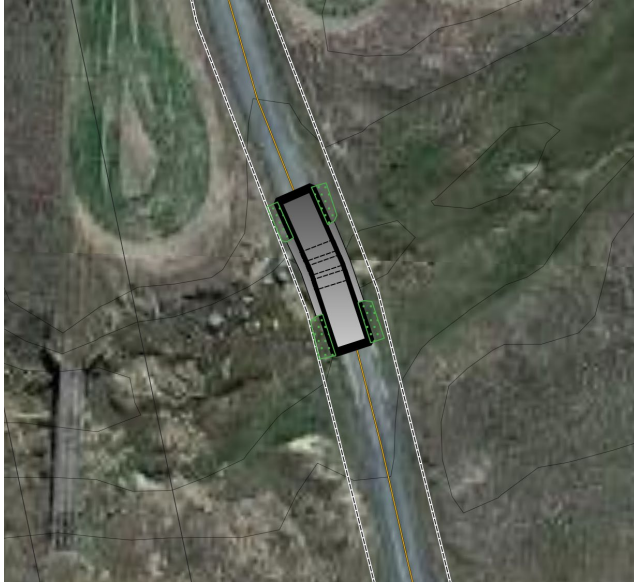
Figure 5-5 Proposed new crossing over Blind Creek. Concrete deck to be approximately 5m wide (Source: Stride Renewables).
