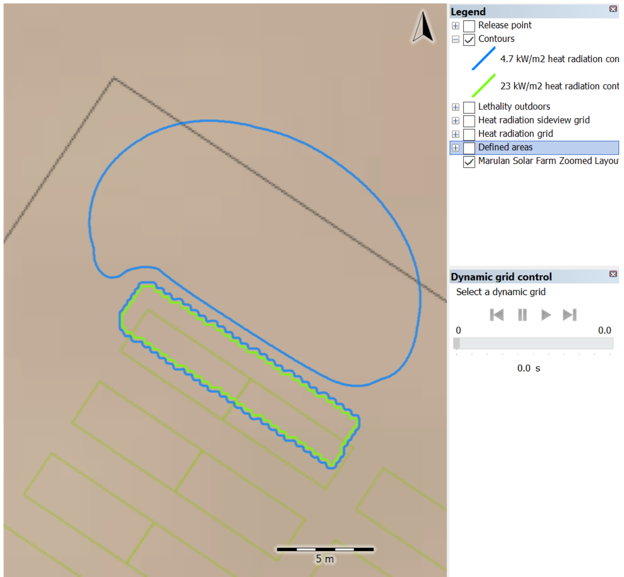
Figure 5-1: Li-Ion Battery Module Fire Radiant Heat Contours
