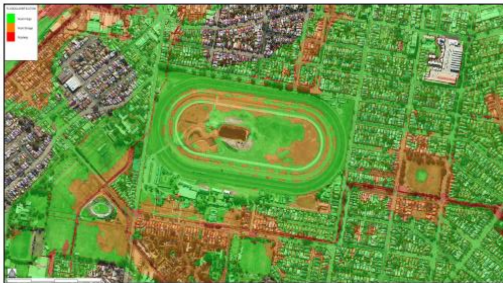
Figure 5: Flood Risk Map with green areas indicating Flood Fringe, orange indicating Flood Storage and red indicating Floodway (Source: CoN Flood Information Certificate FL2019/00101)
