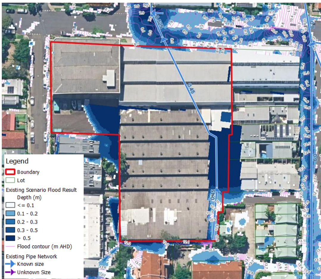
Figure 5.1.1: Existing Condition 1% AEP Flood Depth and Extent
