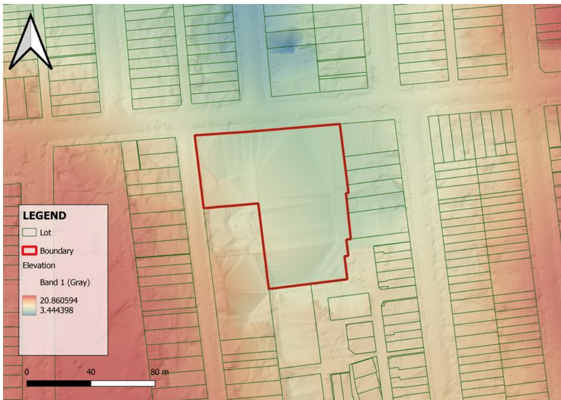
Figure 2.1.1: Site Boundary Location and Topography
