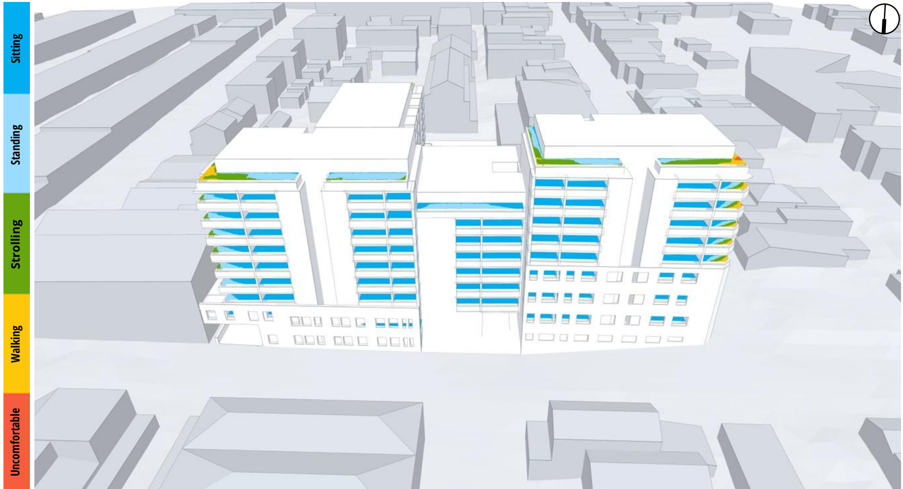
Image 7d: Annual Wind Comfort Conditions – Private Balconies View from North
