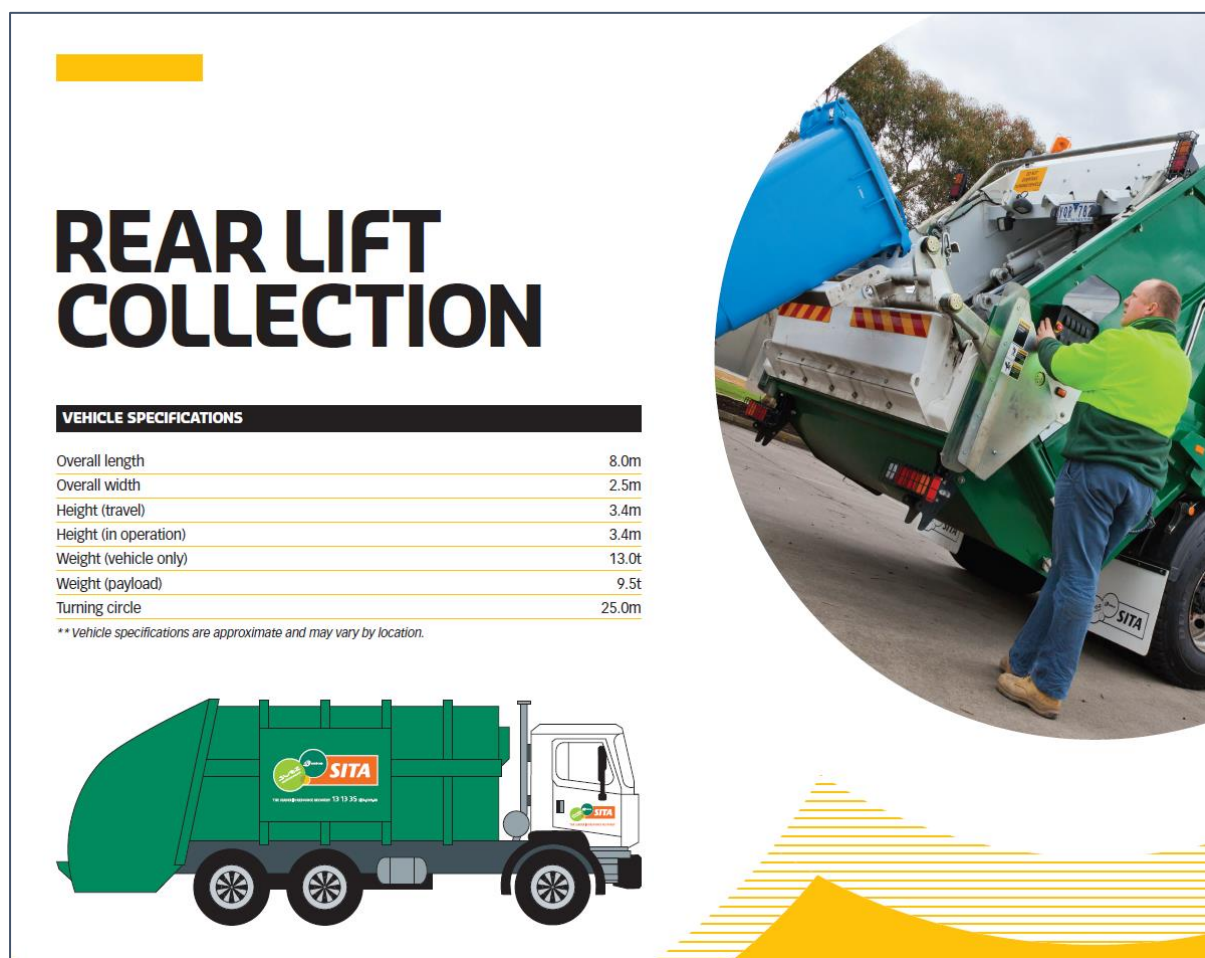
Figure 6.1 – Typical waste truck dimensions (Source: www.sita.com.au )
