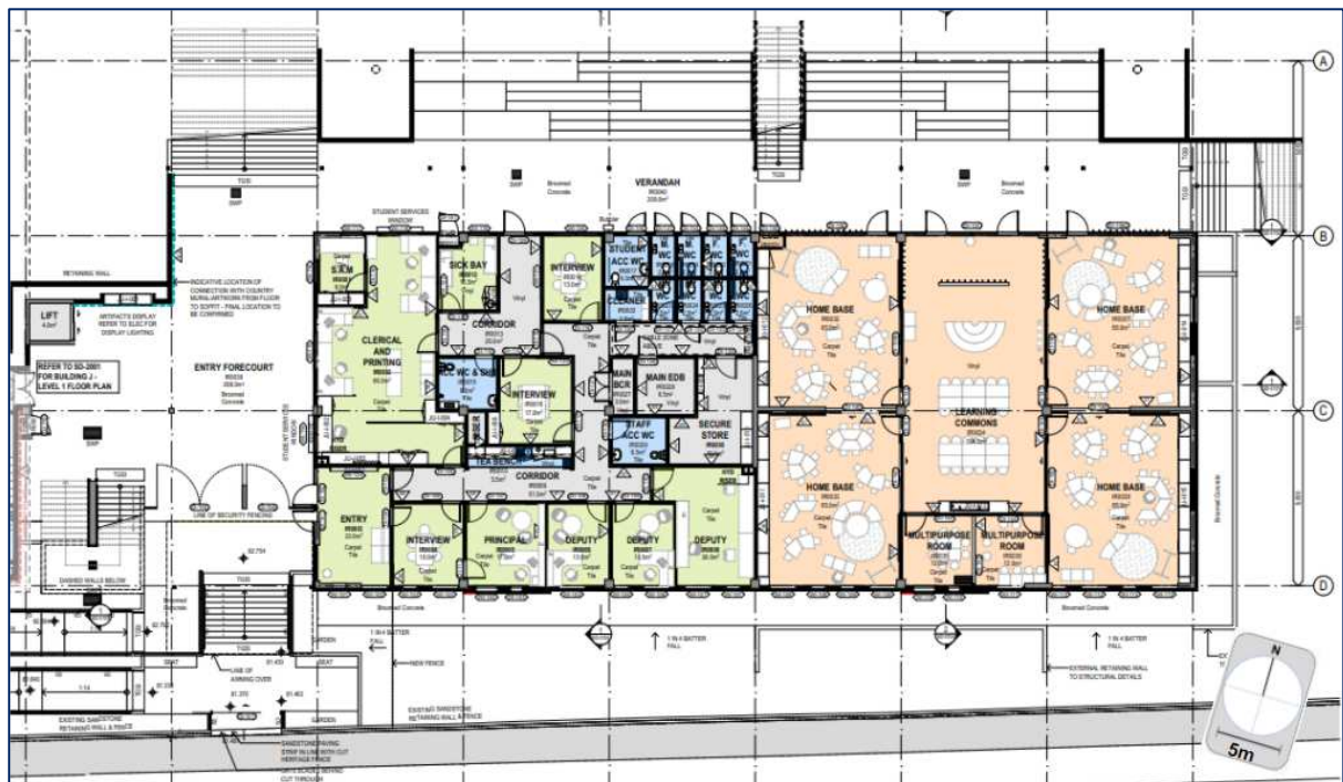
Figure 7 | Building I level 1 floor plan (Source: Applicant's RtS 2021)
