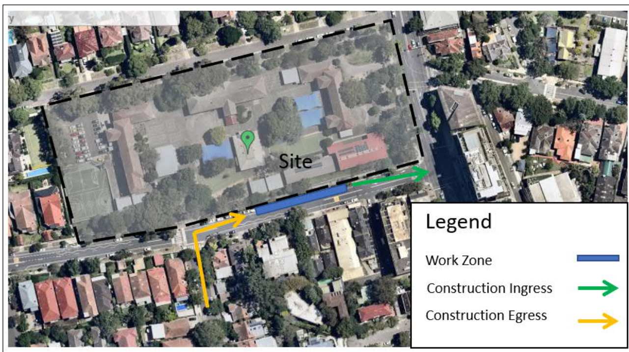
Figure 39: Bay Road Work Zone
