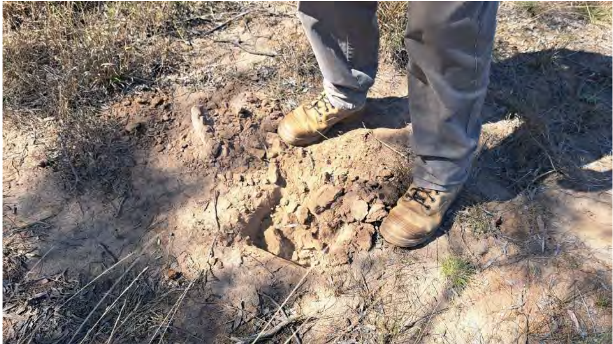
Site 3 - No sand layer present. Appears sheet erosion has stripped all of the A horizon. B Horizon clay layer continues.
