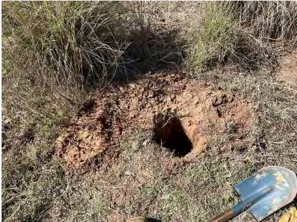
Site 1 - North Section Represented (Excludes gully area). Deep sand to 0.5m, layer continues.
