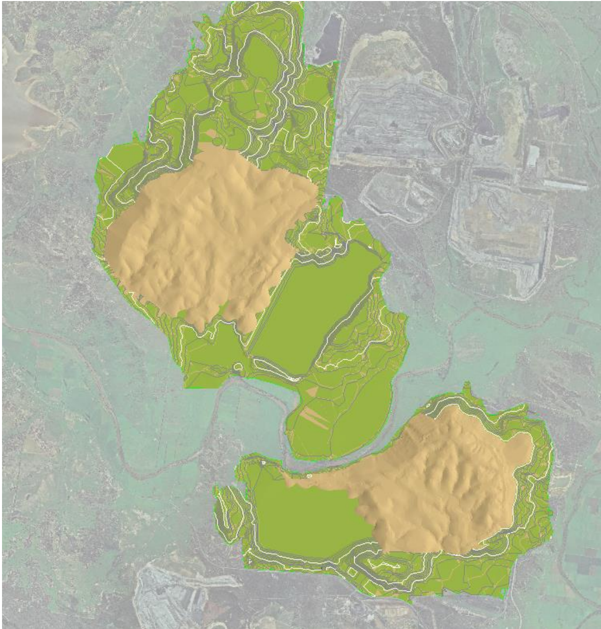
Figure 9: Option 4 – Source Material to Backfill Voids Post-mining
