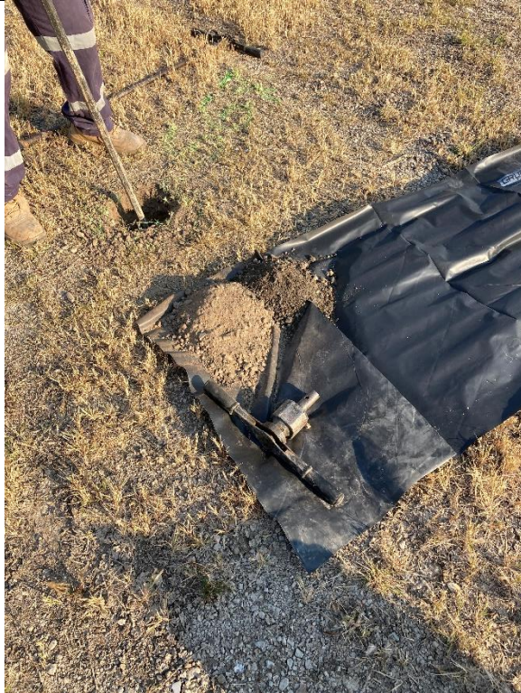
Photograph 1 – Hand auguring before drilling.
