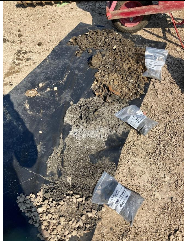
Photograph 6 – Samples were collected from each layer.
