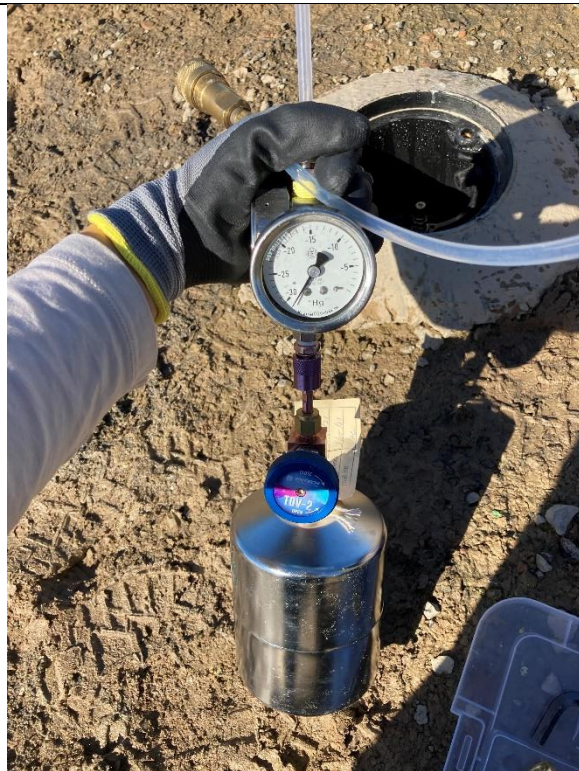
Photograph 17 – Shut-in test (post-sampling).
