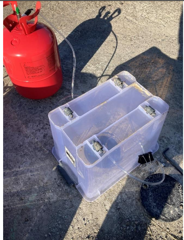
Photograph 14 – Helium test before gas monitoring and vapor sampling.
