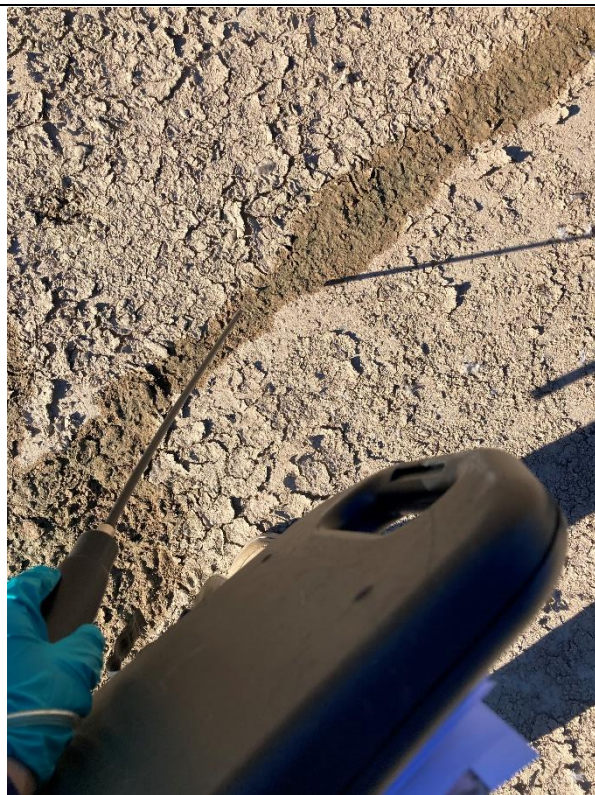
Photograph 29 – Surface gas monitoring.
