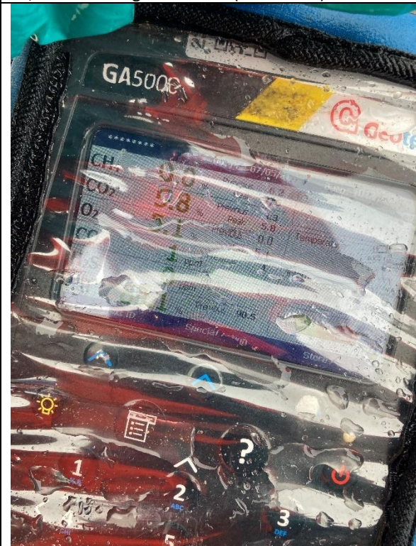
Photograph 15 – Gas monitoring with GA5000.
