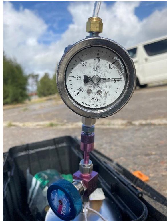
Photograph 18 – Finish sampling and record the end pressure.
