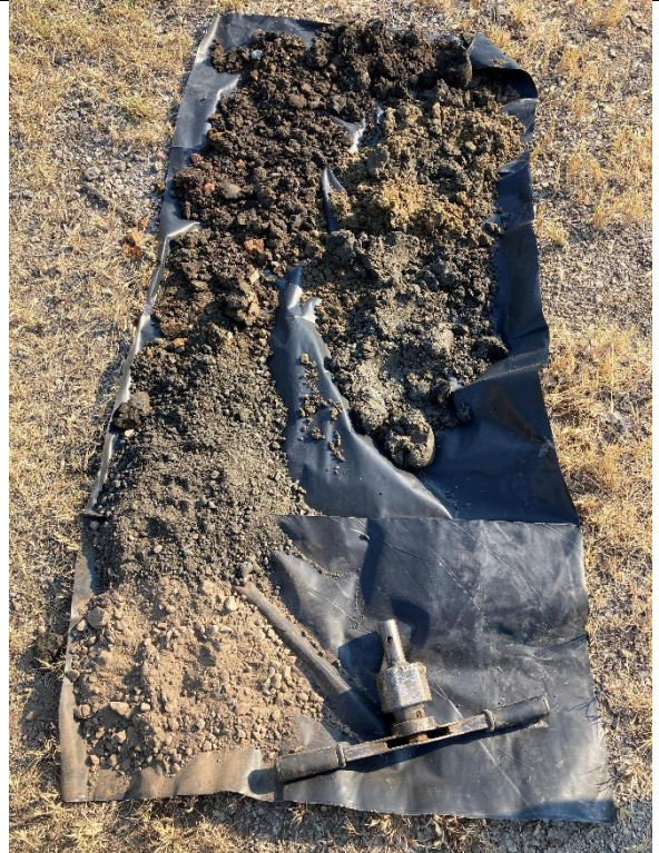
Photograph 2 – Material from the borehole was laid on the plastic sheet for inspection.
