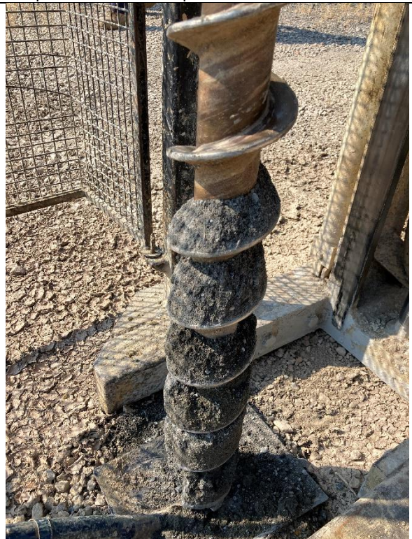
Photograph 4 – Material has strong hydrocarbon odour at GG8 (0.4-0.5 mBGL).
