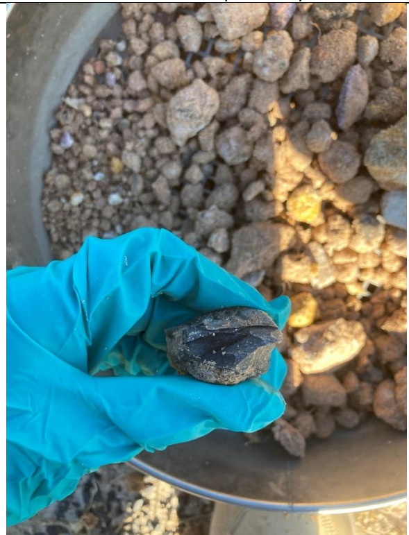
Photograph 26 – Sieve testing – shale and medium to stiff clay cobble was observed.
