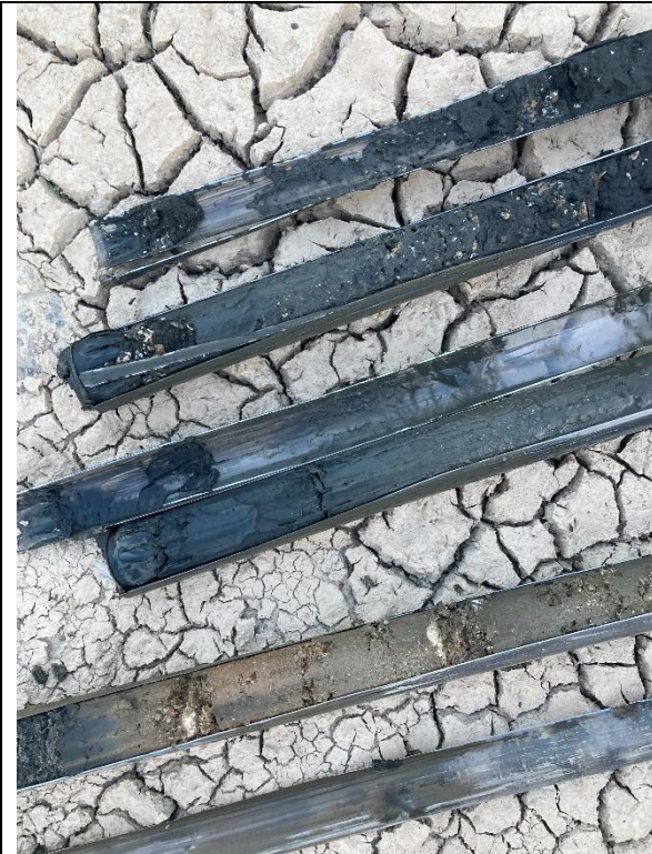
Photograph 13 – Natural high plasticity clay and fill/natural dredged material (with shells).
