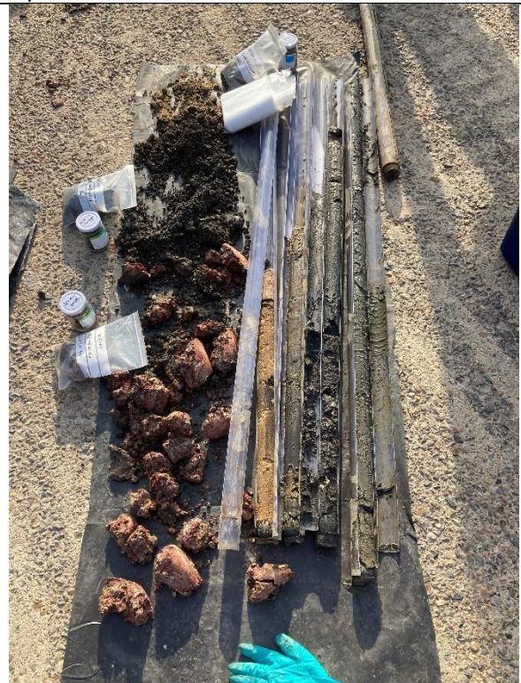
Photograph 8 – Push tubing and sampling after concrete coring at GG5.
