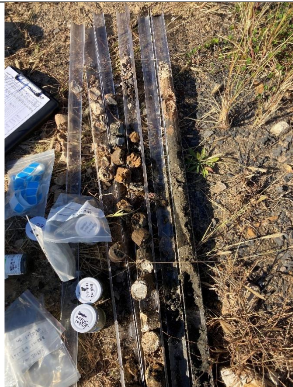
Photograph 12 – Push tubing and sampling at BH8.
