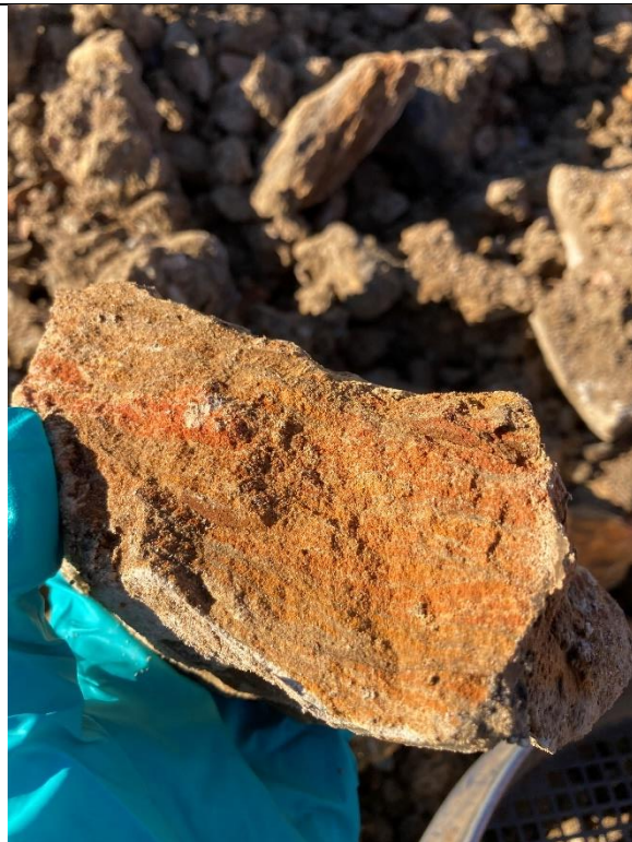
Photograph 25 – Sandstone from the test pit on the soil mound.
