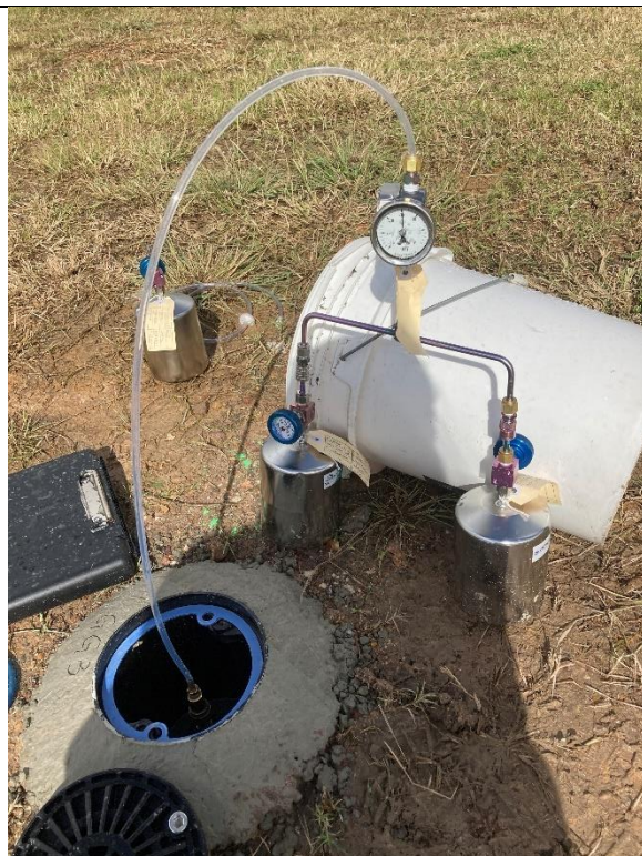
Photograph 19 – Soil vapor primary and duplicate samples.
