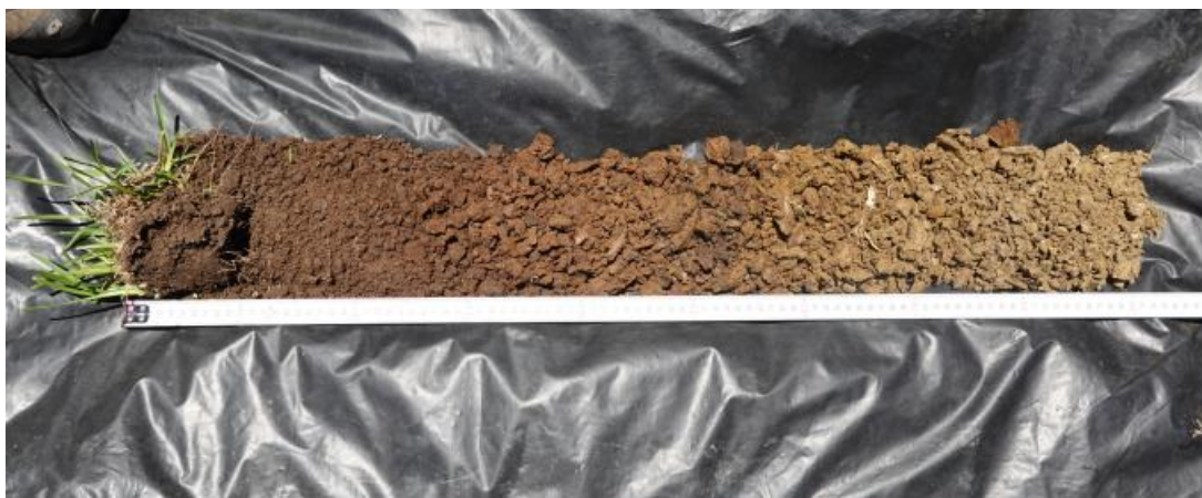
Figure 2.8– Indicative soil sample taken adjacent tree T02. The topsoil was moderately pedaled medium to light clay over a subsoil structure of strongly pedaled heavy clay. (Photo: Arterra 24/01/25)
