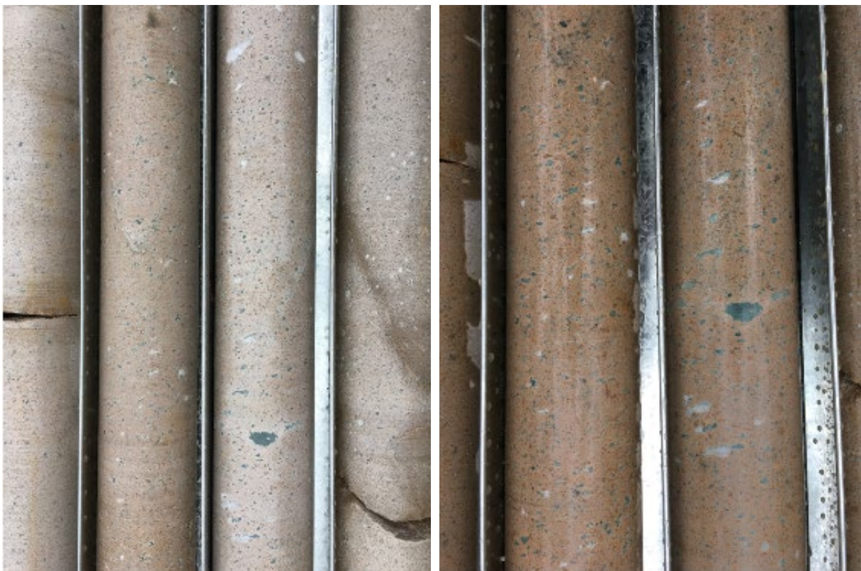
Photograph 3: DCQ DDH19 Rock Core sample when dry and then wet, showing the good aesthetic values of the material.
