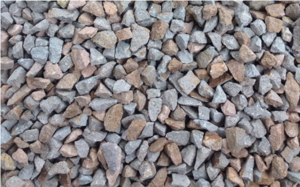
Photograph 4: DCQ 20 mm aggregate (from a laboratory crushed core sample).
