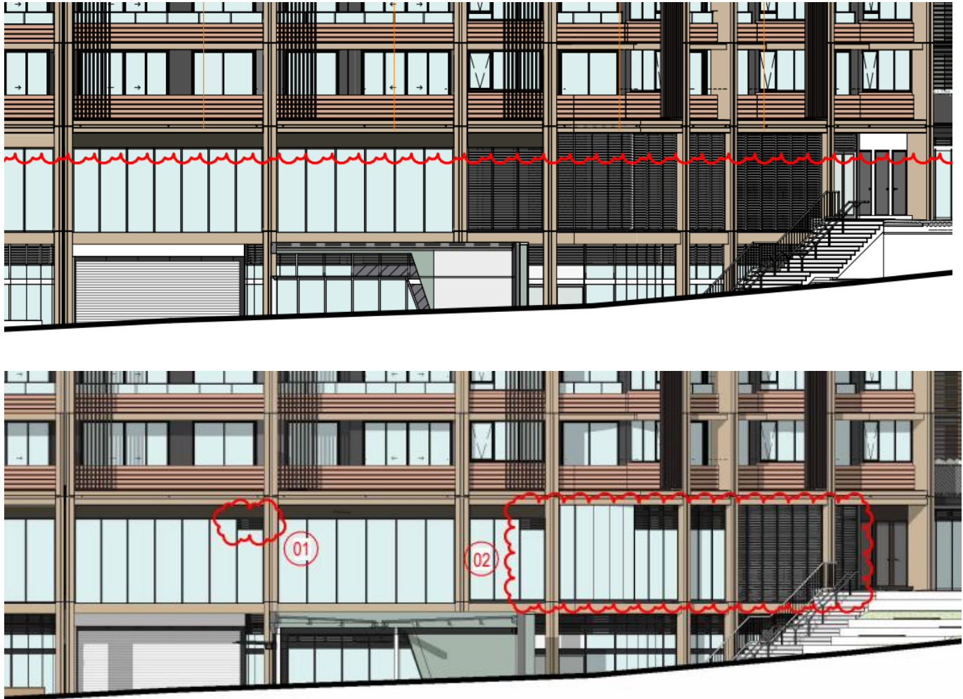
Figure 4 Amendments to community facility louvre locations at Tower B north west elevation – as approved (top) and as amended (bottom)
