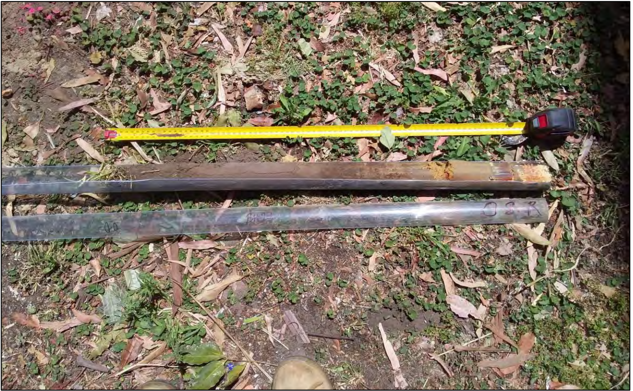
Photograph 7. Soil profile depicting the fill / natural matrices encountered within BH21 (0.0-0.8 m). Date: 01.12.2020.
