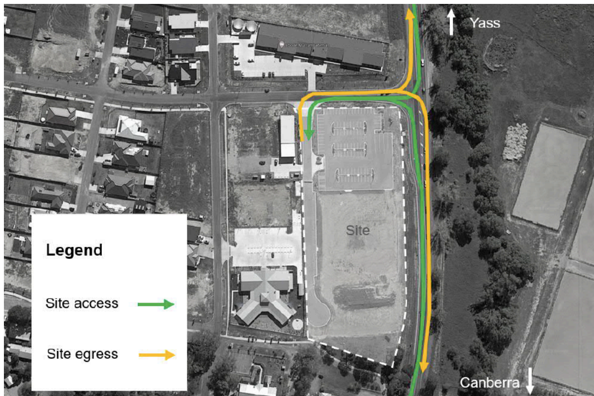
Figure 7-14 Construction vehicle haulage routes
