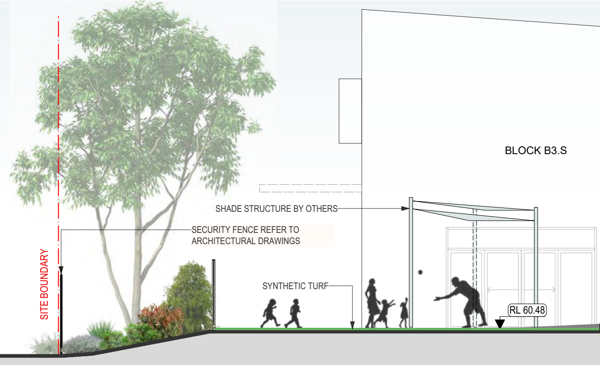
SECTION 2: DEERUBBIN DRIVE / BUILDING B3.S SCALE: 1:50 @A1
