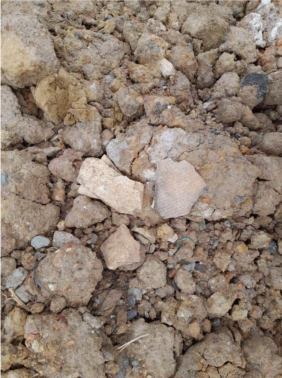
Photograph 2. Fibre cement containing chrysotile, amosite and crocidolite asbestos encountered within subject stockpile. Date: 09/10/2024.
