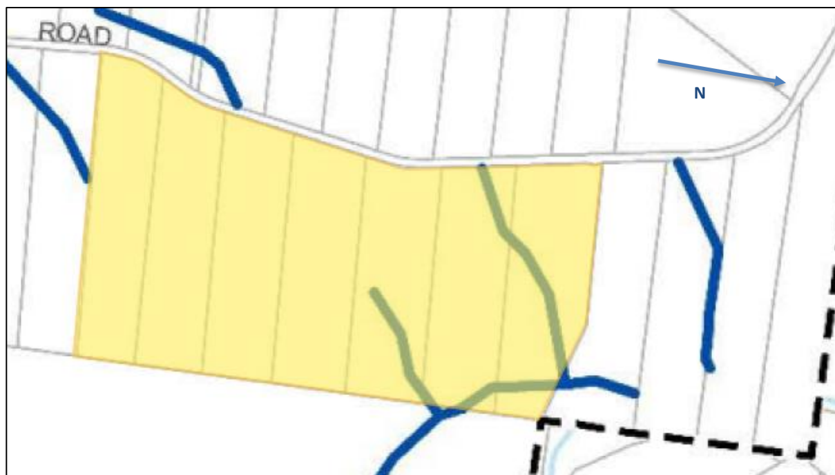
Figure 6 Indicative trunk drainage paths (N.T.S)
