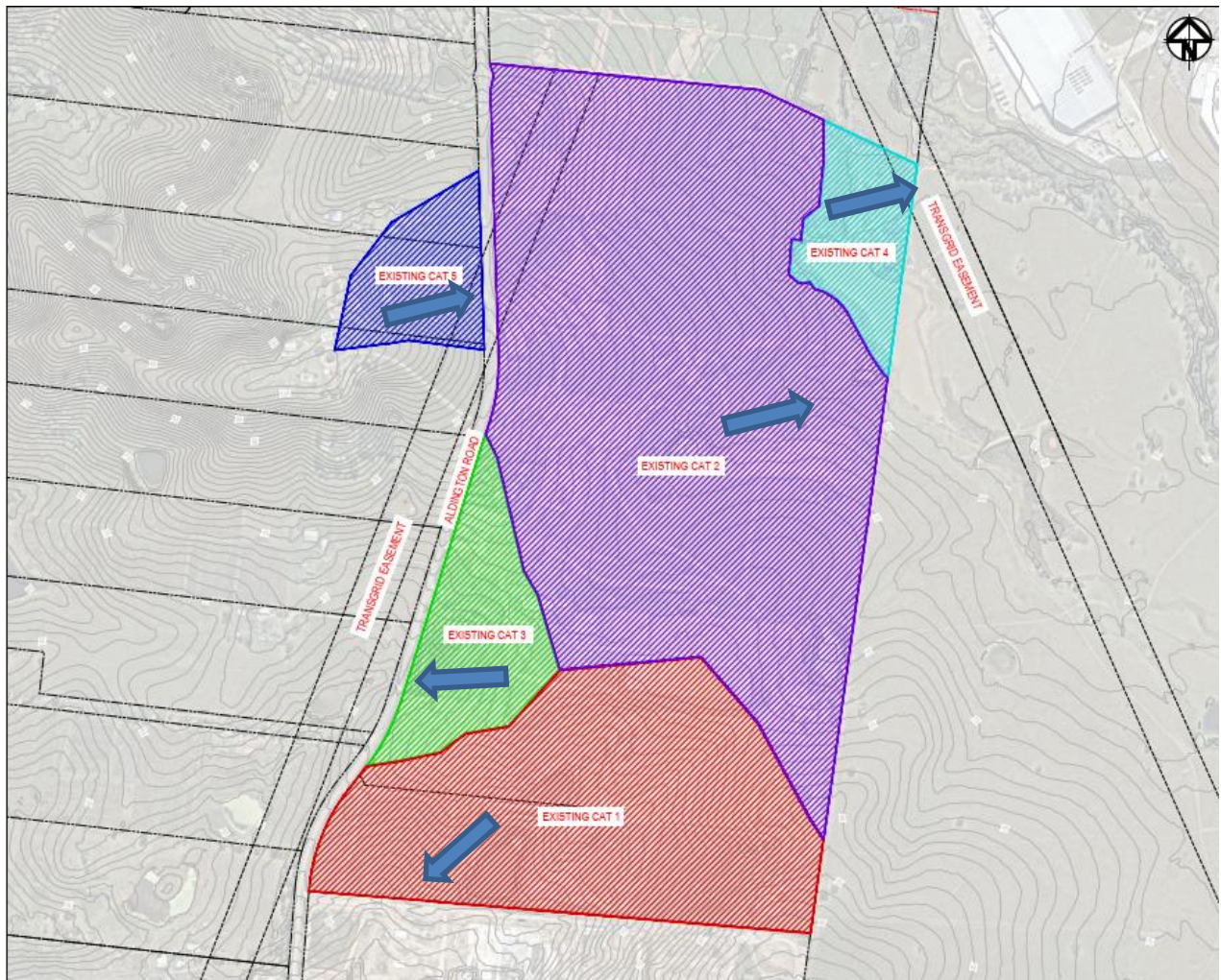
Figure 5: Catchment delineation under pre-development conditions
