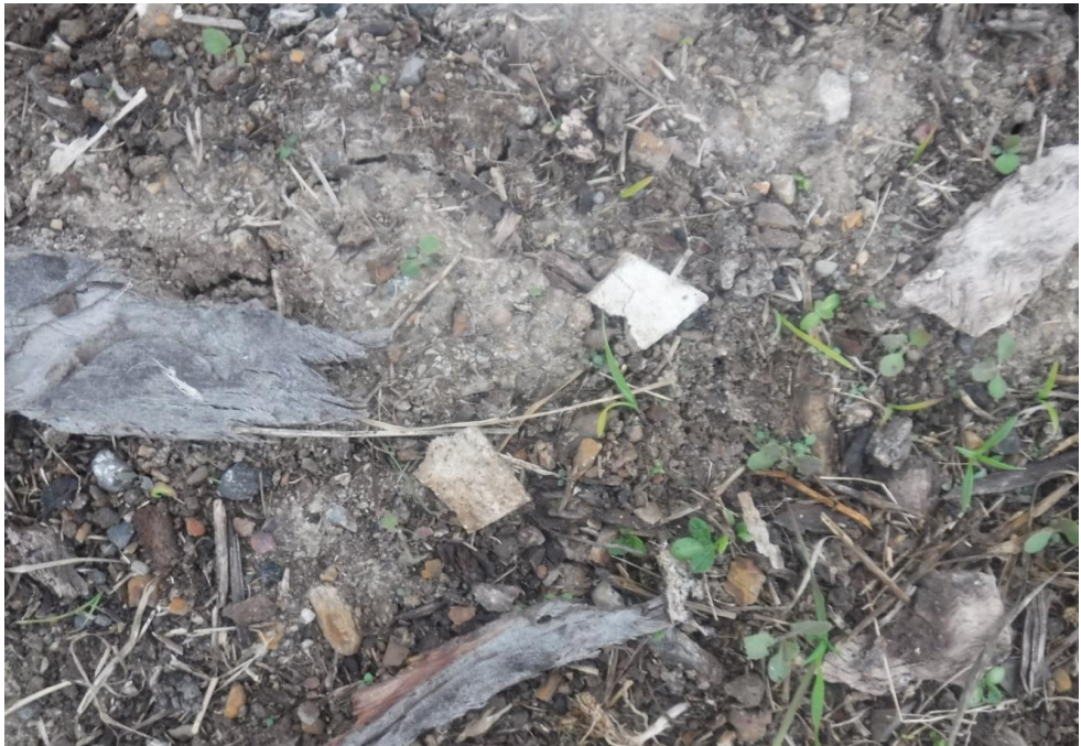
Photo 8: Multiple fragments of ACM were observed on the surface of fill in the central stockpile are in Lot 22
