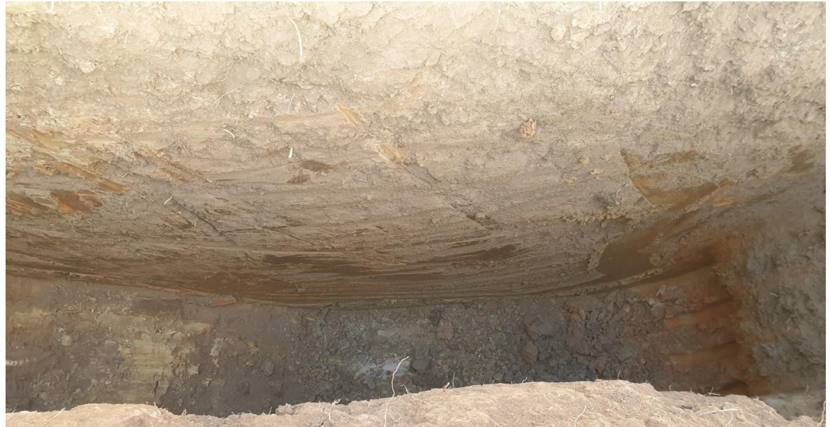
Photo 26: Fill in the dam wall in the east of Lot 22 (TP18)
