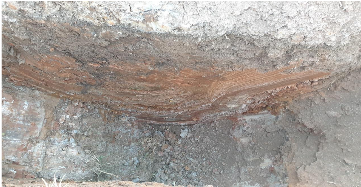
Photo 27: Fill within a fill platform in the centre of Lot 22 (TP10)
