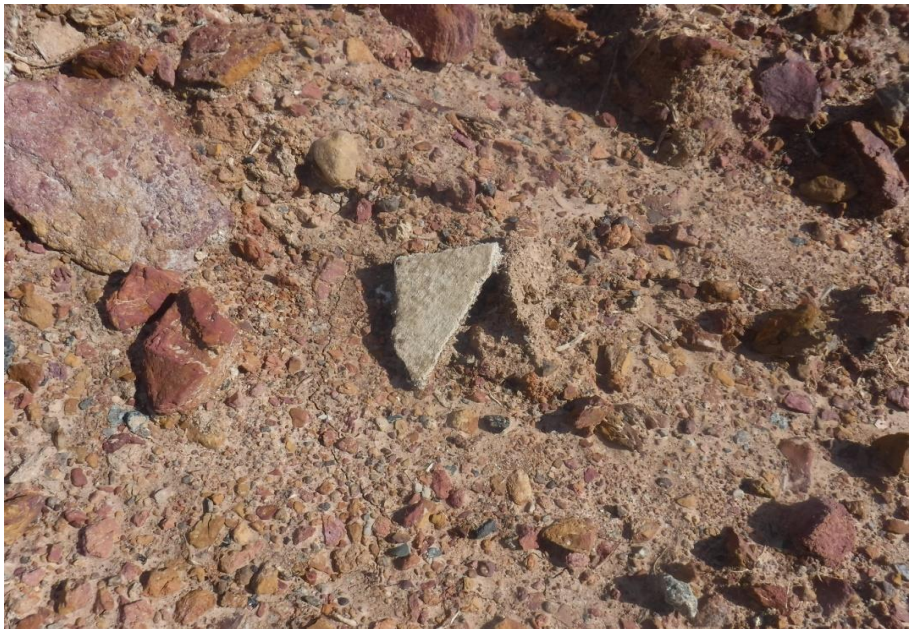
Photo 19: Fragment of ACM on the surface of a stockpile in the southeast
