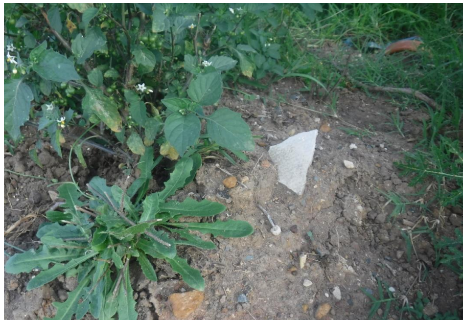
Photo 27: ACM fragment on the surface of the soil stockpile in the southwest.
