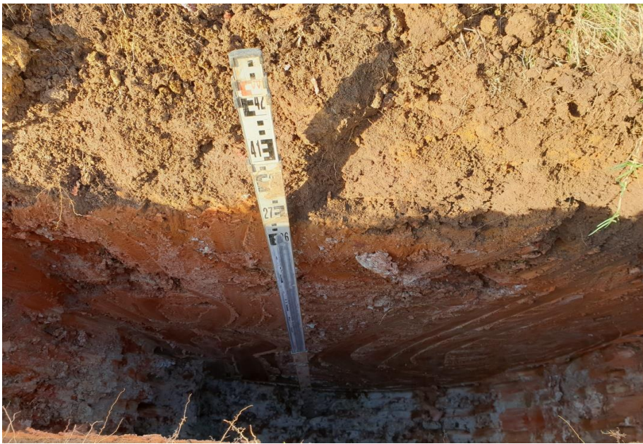
Photo 37: Filling overlying natural clays at TP9
