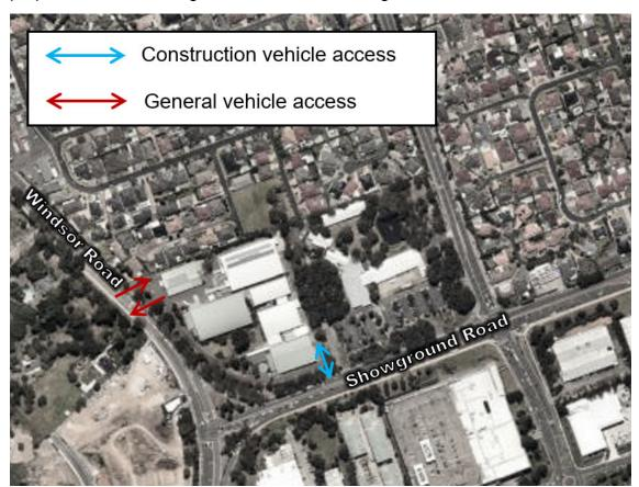
Figure 25 Construction vehicle site access
