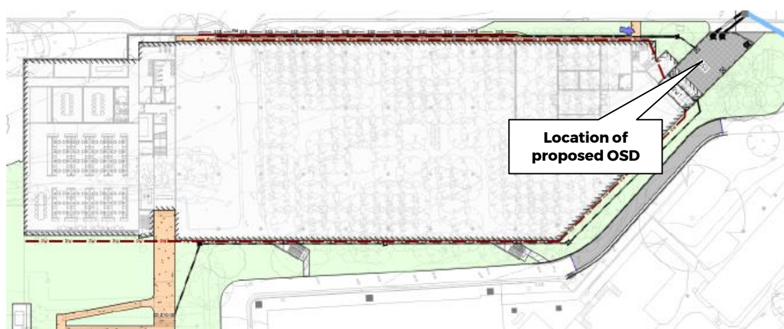
Figure 22: Proposed OSD & Rainwater Tank Location Source: Northrop Stormwater Management Report
