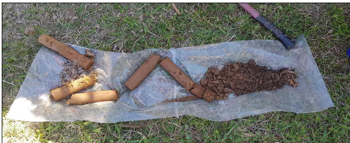
**Image 7.2.1 Example of soil profile at BH04, from surface (right) to underlain natural material (left)**
