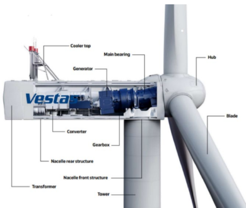
Figure 10 | Vestas wind turbine nacelle components
