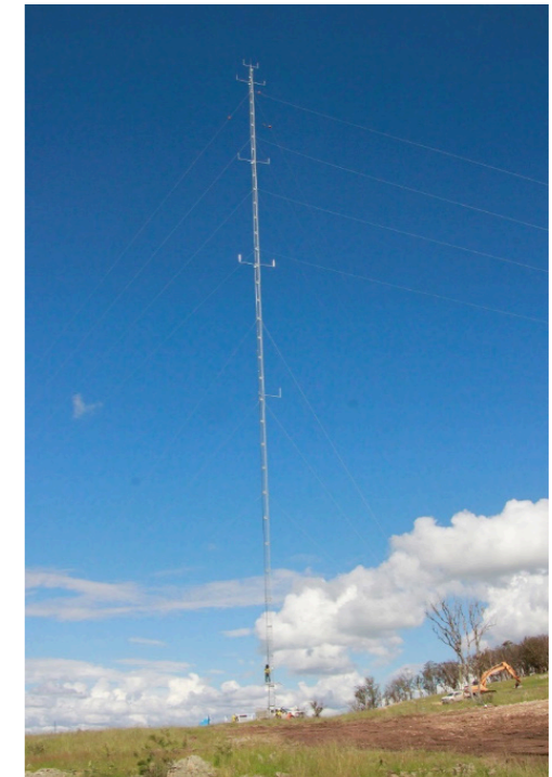
Image 7: Meteorological monitoring masts (Source: Vestas)
