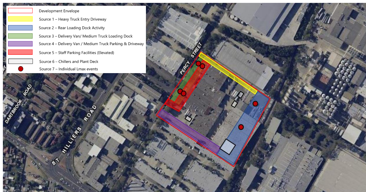
Figure 15. Noise Sources from Acoustic Report (20200597.1/2005A/R7/WY) (Source: Acoustic Logic, 2021)
