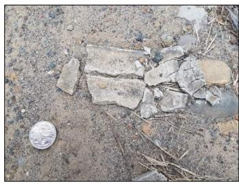
Plate 20 – Asbestos fragments on northeast boundary of 11-13 Percy Street (North gate).
