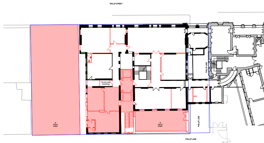
Demolition Plan - Level 2
