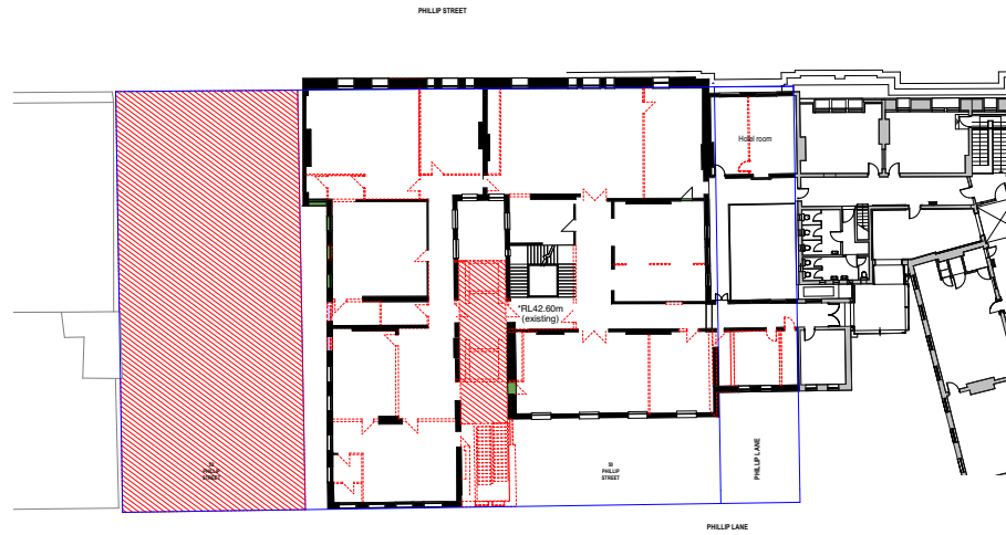
Demolition Plan - Level 5
