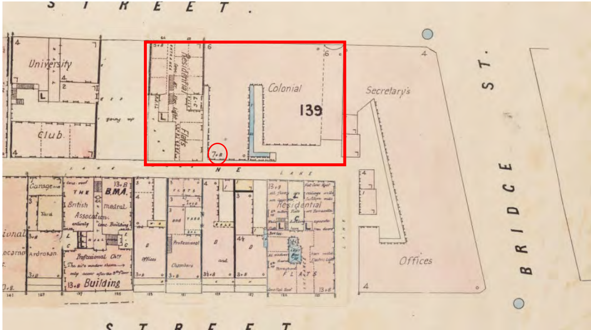
Figure 3-26 Plan of the study area in the 1892-1937. Note the notation circled in red for 50 Phillip indicating the presence of a basement in at the east end of the structure (i.e. "B"). (Source: Ignis et Aqua series Sheet 46.ML Z/MAXX 811.17/1892/1 FM4/10537)
