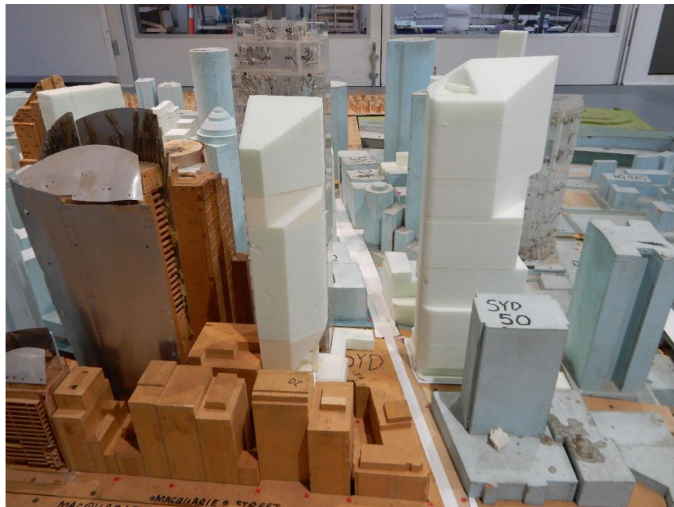
Figure 5 – Close-up view from the east of the 1/400 scale Proposed Configuration model of the 50 Phillip Street Development in the wind tunnel.
