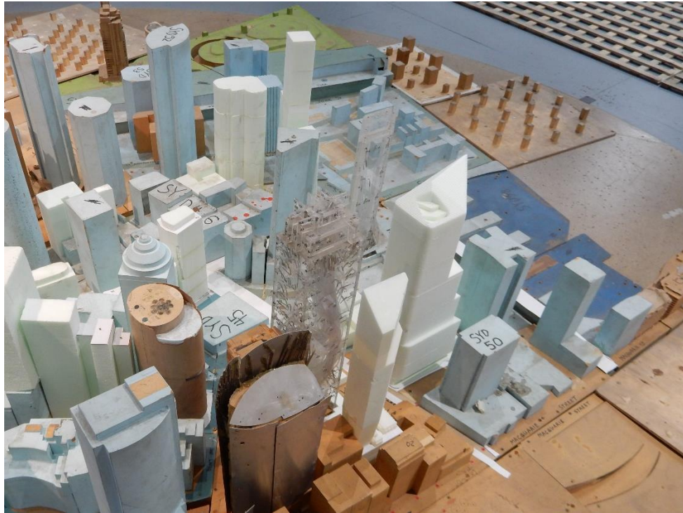
Figure 4 – View from the southeast of the 1/400 scale Proposed Configuration model of the 50 Phillip Street Development in the wind tunnel.
