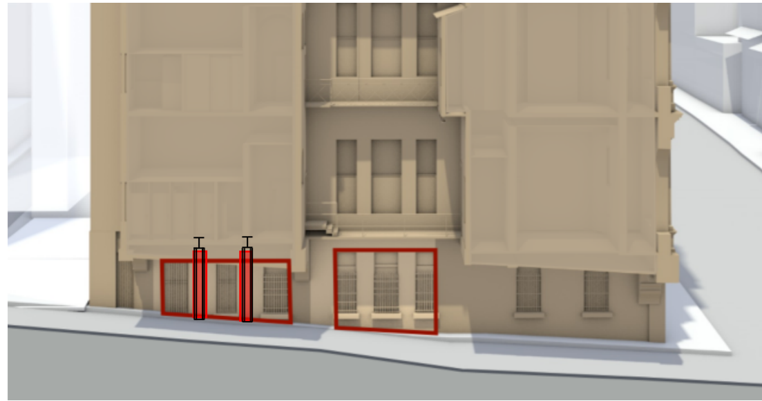
ELEVATION OF WORKS LOCAL DEMOLITION OF PIERS
