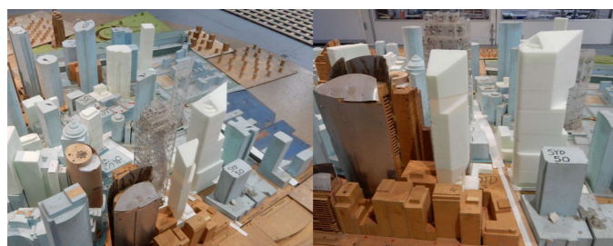
1/400 scale Proposed Configuration model of the 50 Phillip Street Development in the wind tunnel
