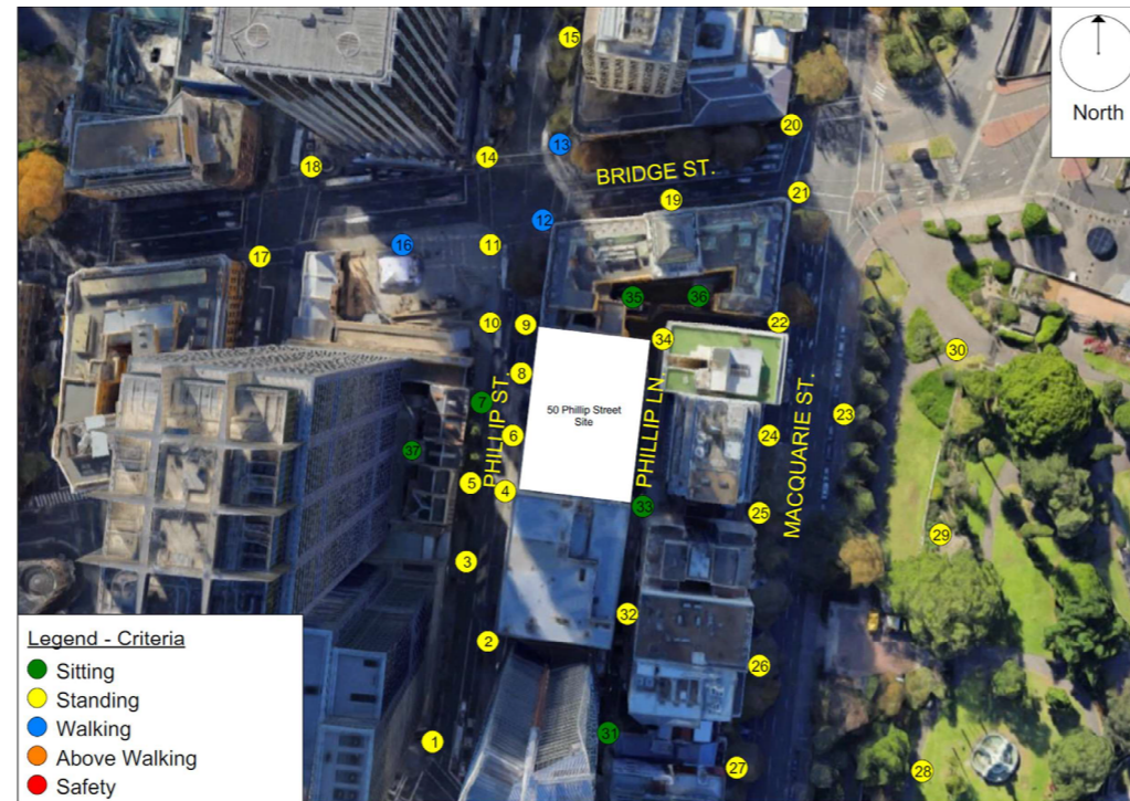
Summary of Ground Level wind conditions for the Proposed Configuration for 360 degrees of wind direction
