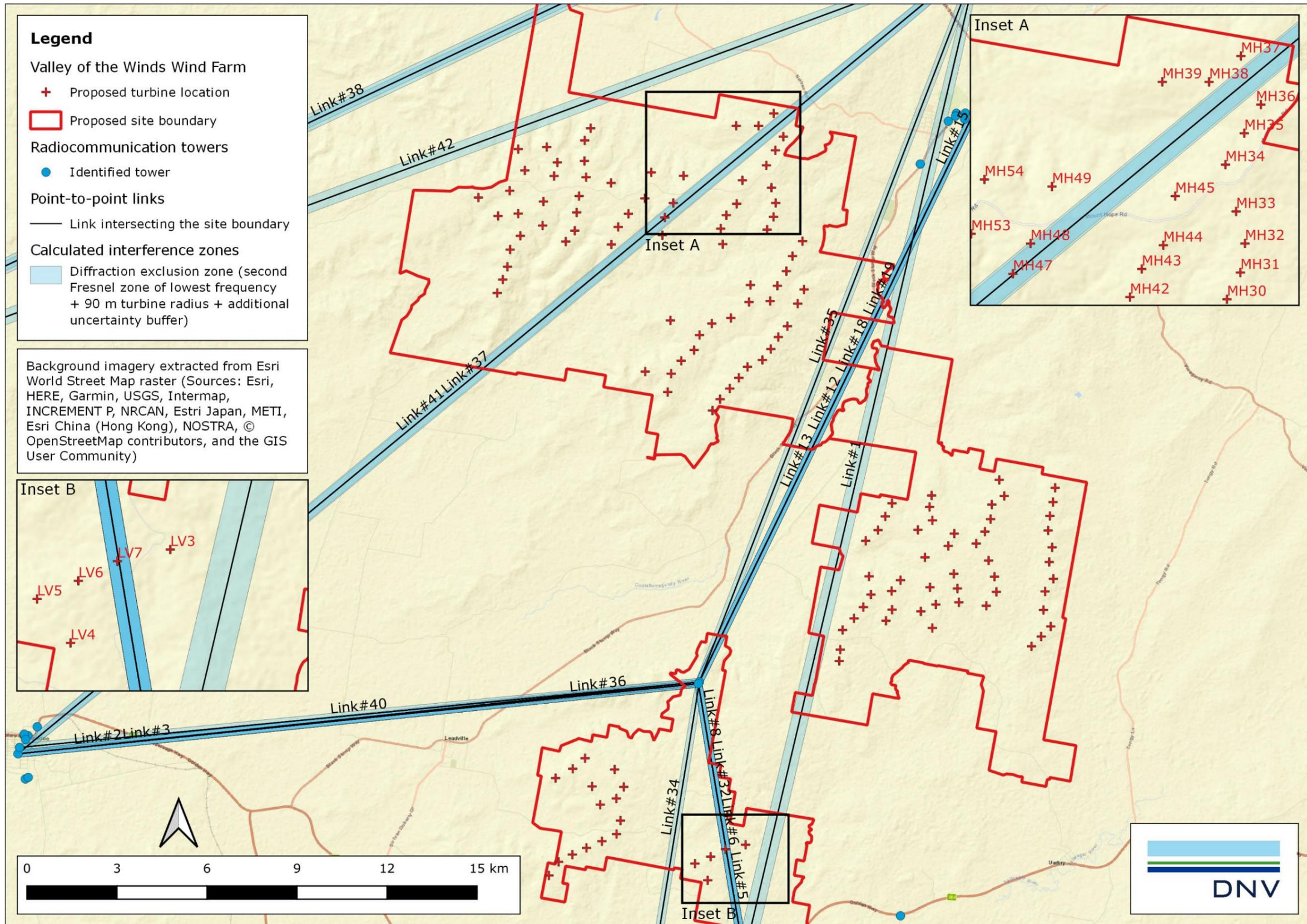
**Figure 8 Identified point-to-point radiocommunication vectors crossing the proposed Project and calculated interference zones**
