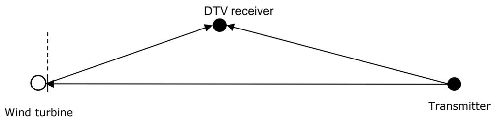
**Figure A.2 Back scatter signal path for DTV signals**
