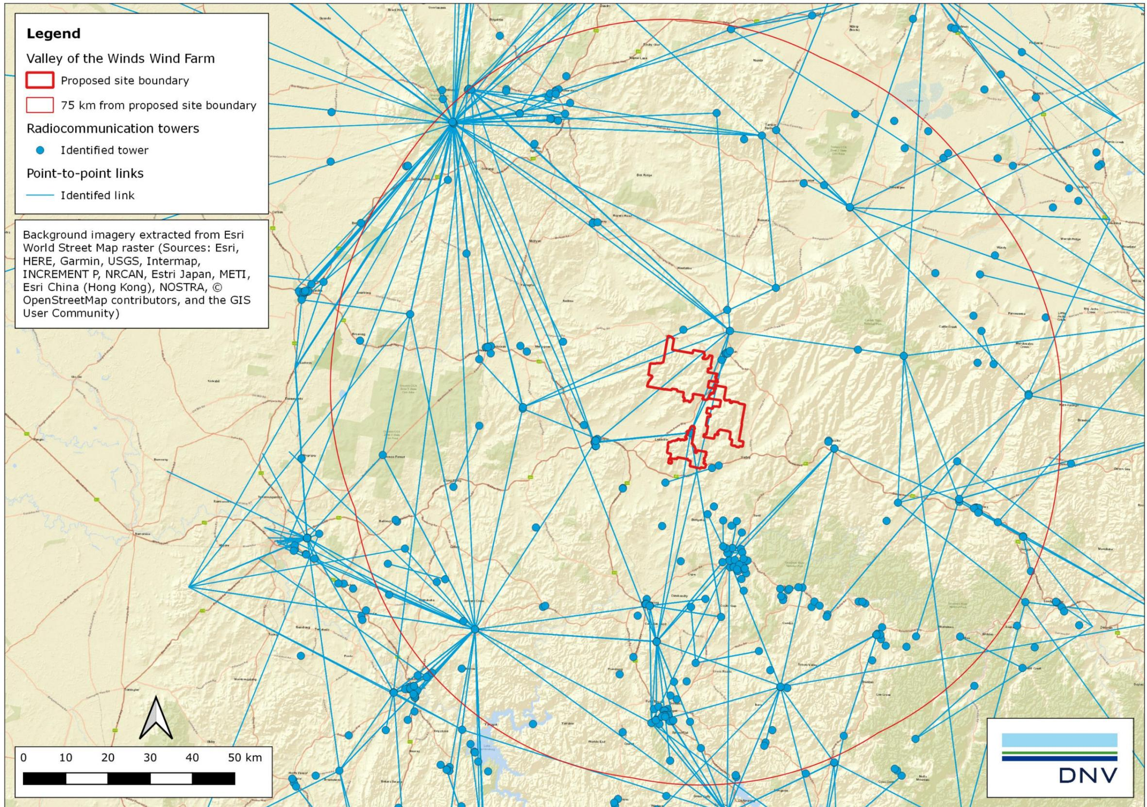
**Figure 7 Identified transmission vectors for fixed licences of point-to-point type in the vicinity of the proposed Project**
