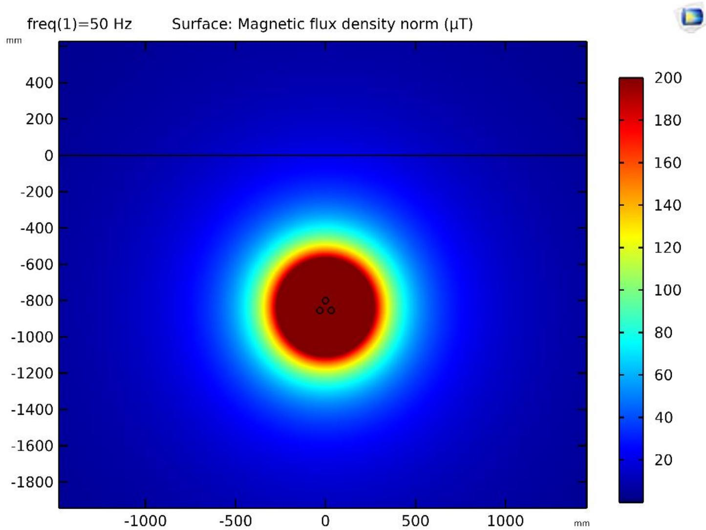
**Figure 2 Magnetic field ( $\mu\text{T}$ ) distribution around the cable at 800 mm below ground level under worst-case conditions**
