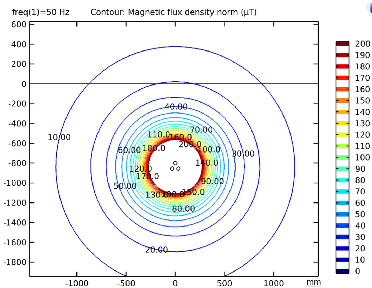
**Figure 3 Magnetic field ( $\mu\text{T}$ ) contours around the cable at 800 mm below ground level under worst-case conditions**
