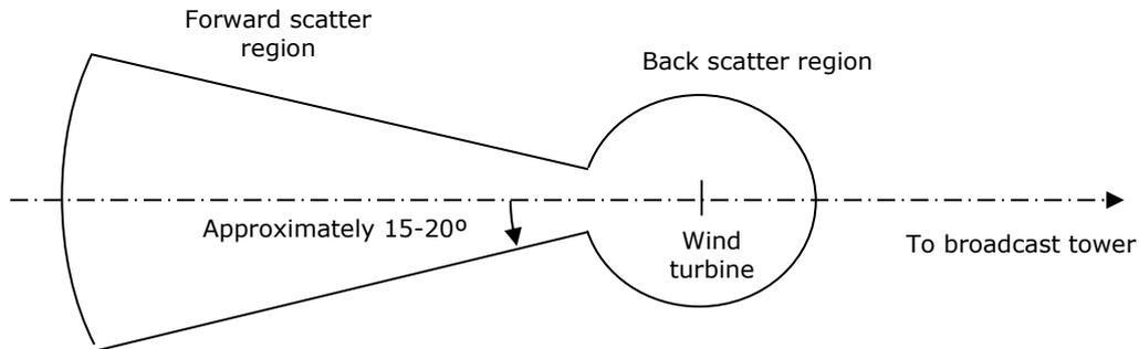
**Figure A.3 Potential television interference zones around a wind turbine**
