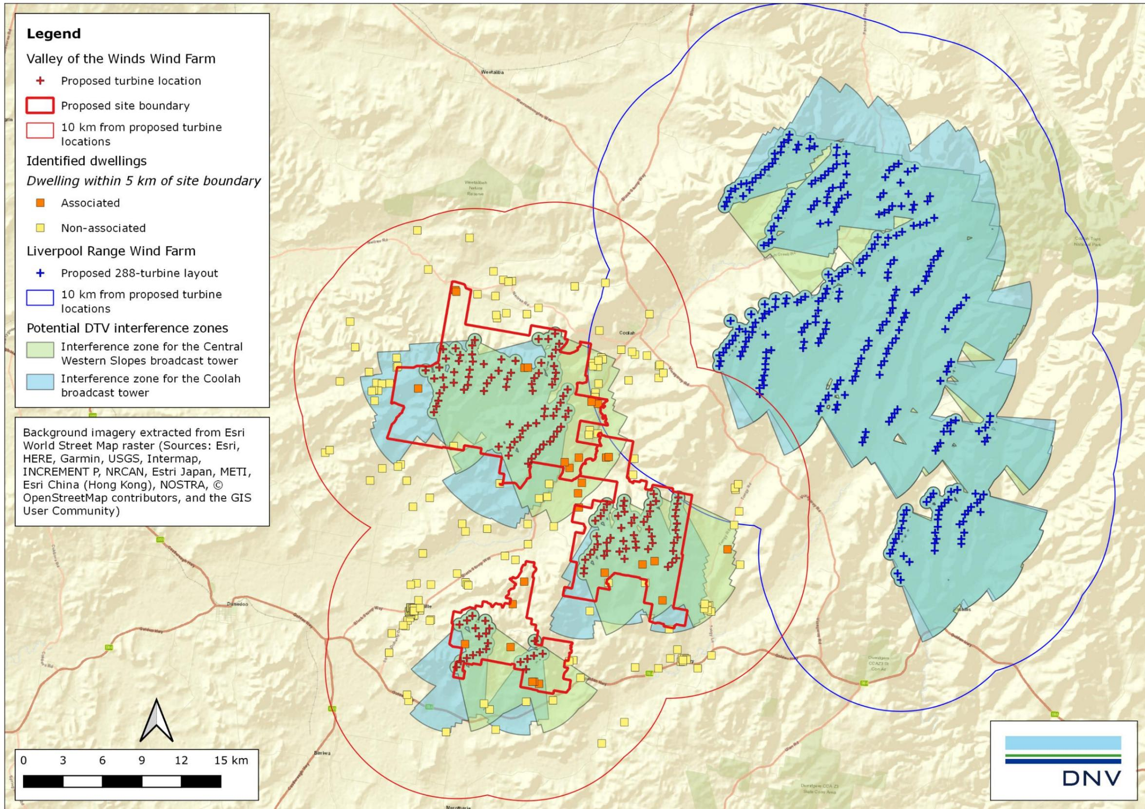
**Figure 24 Potential cumulative EMI impacts to television signals from the Central Western Slopes and Coolah broadcast towers**
