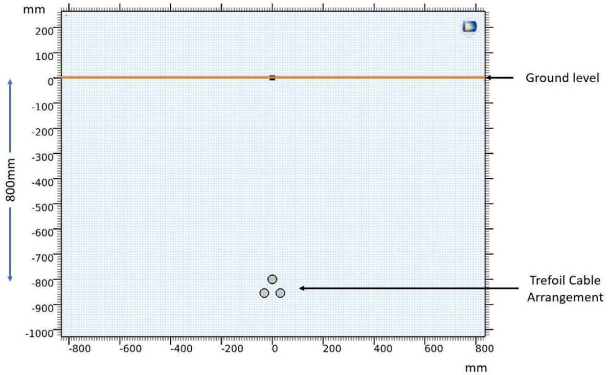
**Figure 1 Underground cable arrangement and burial depth**
