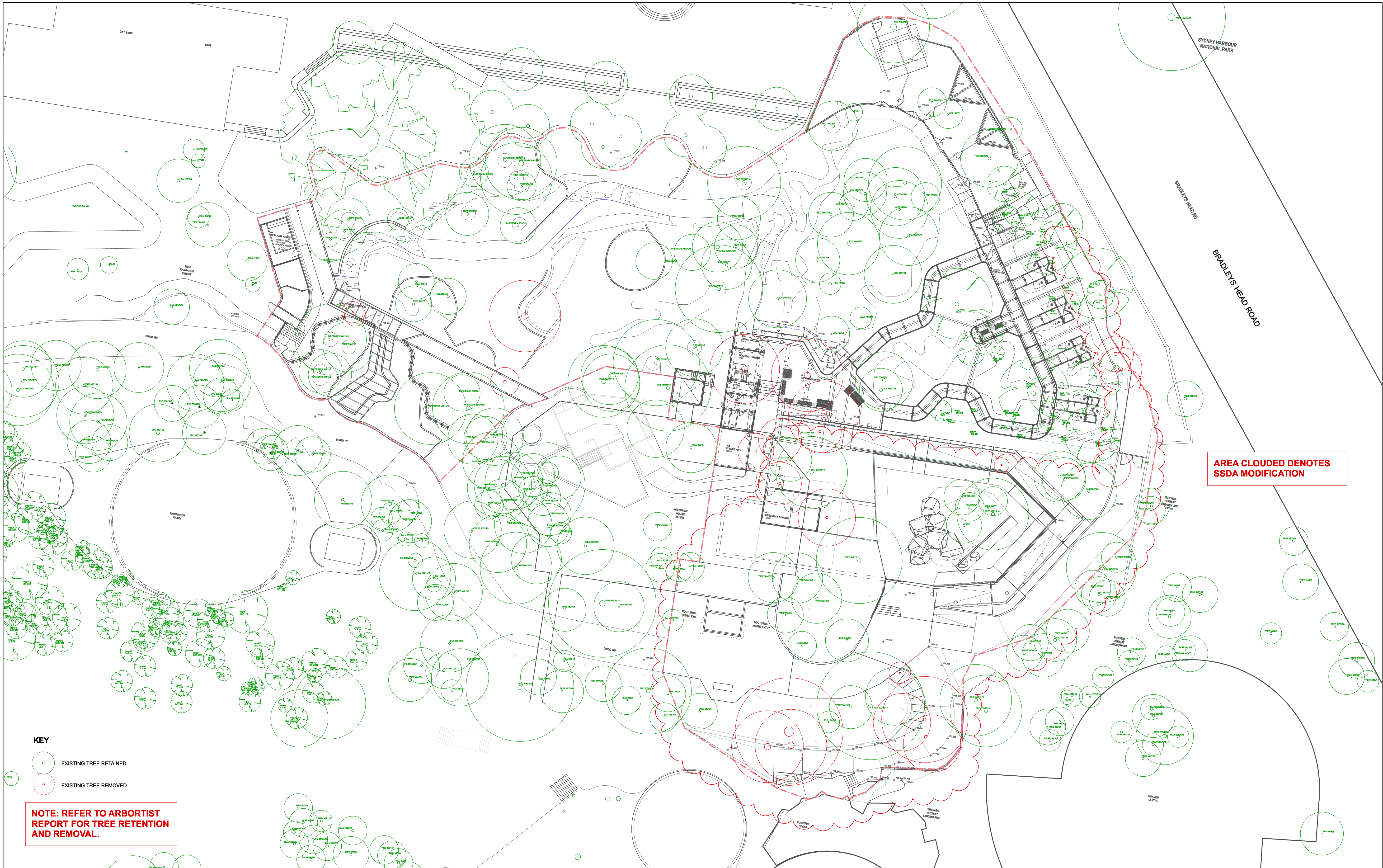
1 TREE PROTECTION AND REMOVAL PLAN 1:250
