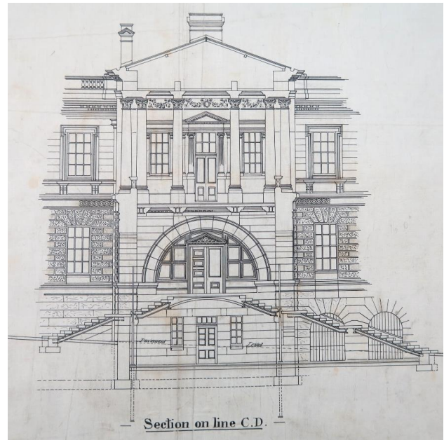
Figure 208 – Section C-D of Link Building (generally as constructed) showing the eastern façade of the Link Building behind the front portico
