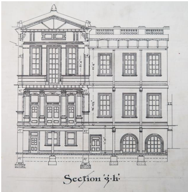
Figure 207 – Section G-H of Link Building (generally as constructed) showing the internal face of the eastern facade
