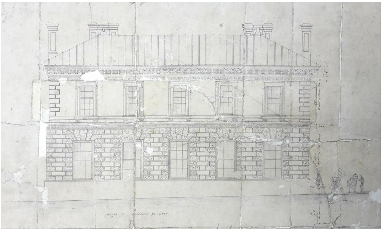
Figure 166 – Elevation of Treasury Building, facing Bridge Street, c. 1850 (not built as drawn – built instead with seven window bays and a door to Bridge Street)
