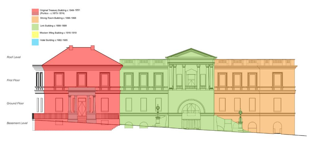
Figure 16 – Extract of 'as built' plans showing period of construction – Macquarie Street elevation Source: Hassell Architects with Urbis annotations and overlay
