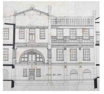
Figure 233 – Section G-H of Link Building (generally as constructed) showing the internal face of the eastern facade
