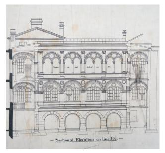
Figure 232 - Section J-K of Link Building (generally as constructed) showing the exterior face of the arcade
