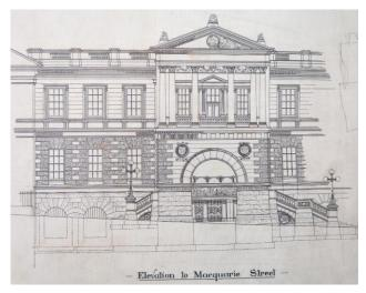
Figure 228 – Eastern elevation to Macquarie Street of Link Building (generally as constructed)
