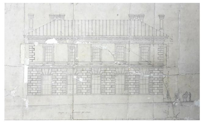
Figure 189 – Elevation of Treasury Building, facing Bridge Street, c. 1850 (not built as drawn – built instead with seven window bays and a door to Bridge Street)
