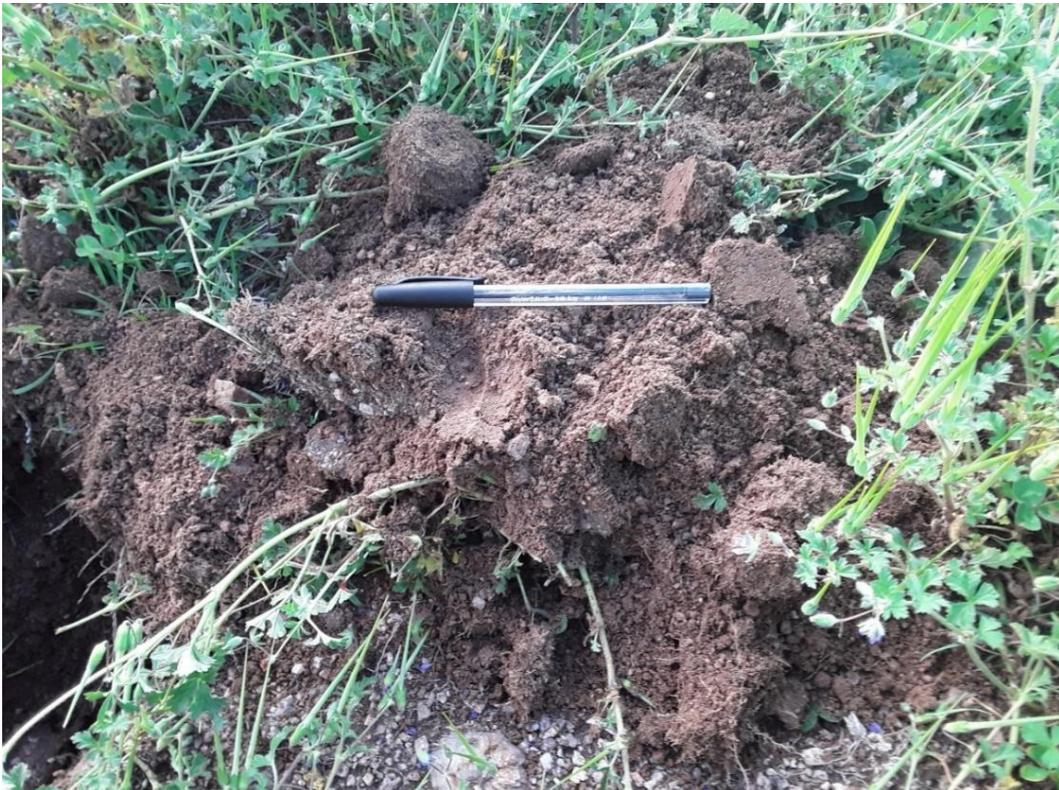
Photo 9-6: Typical shallow soil profile with brown, coarse grained, loamy sand, (no cohesive fines) to 500mm in the study area
