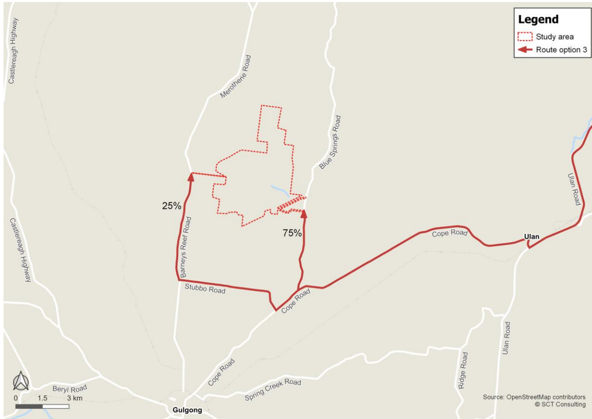
Figure 3–3 Construction traffic distribution – option 3 for heavy vehicle access to the north portion
