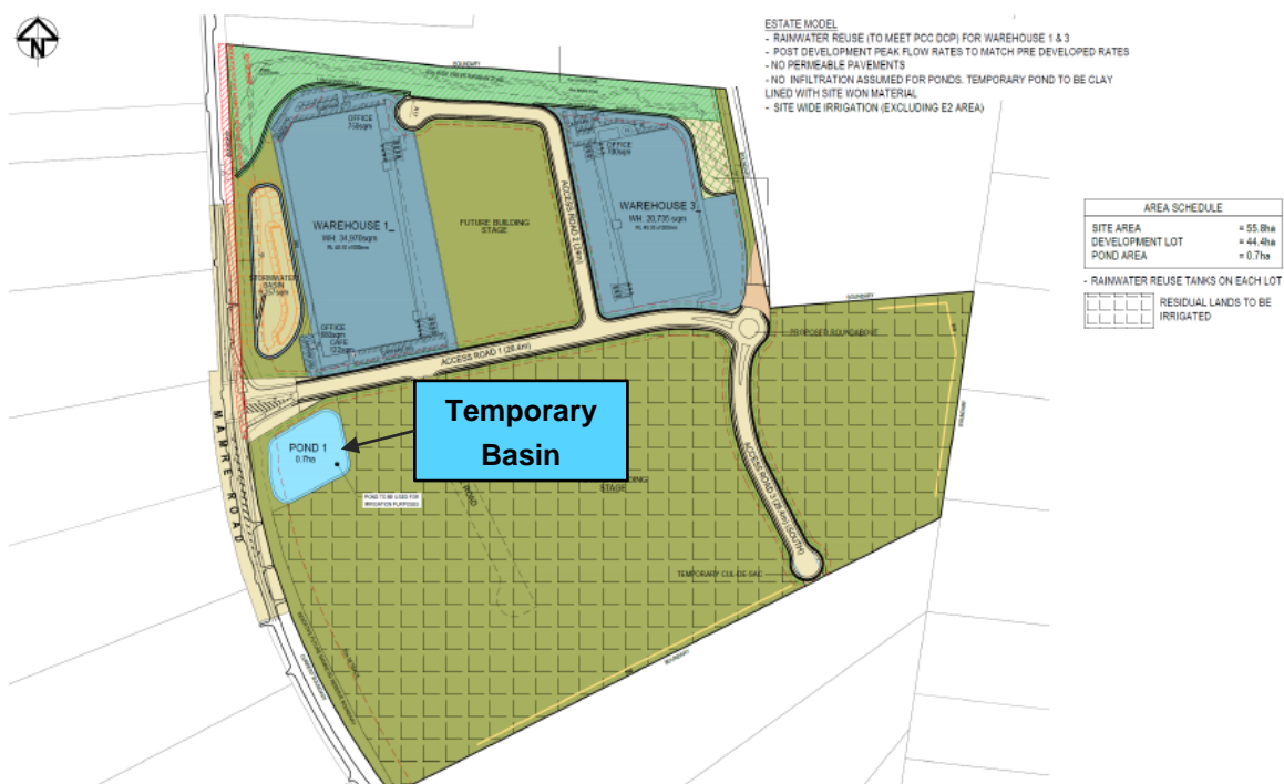
Figure 10 | Approved Stage 1 development stormwater management system
