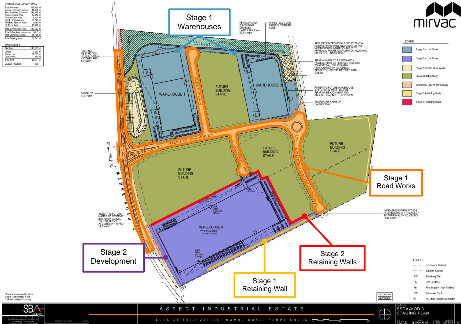
Figure 6 | Proposed Staging Plan
