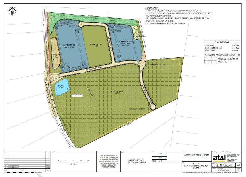
Figure 5: Stage 1 Stormwater Management Plan
