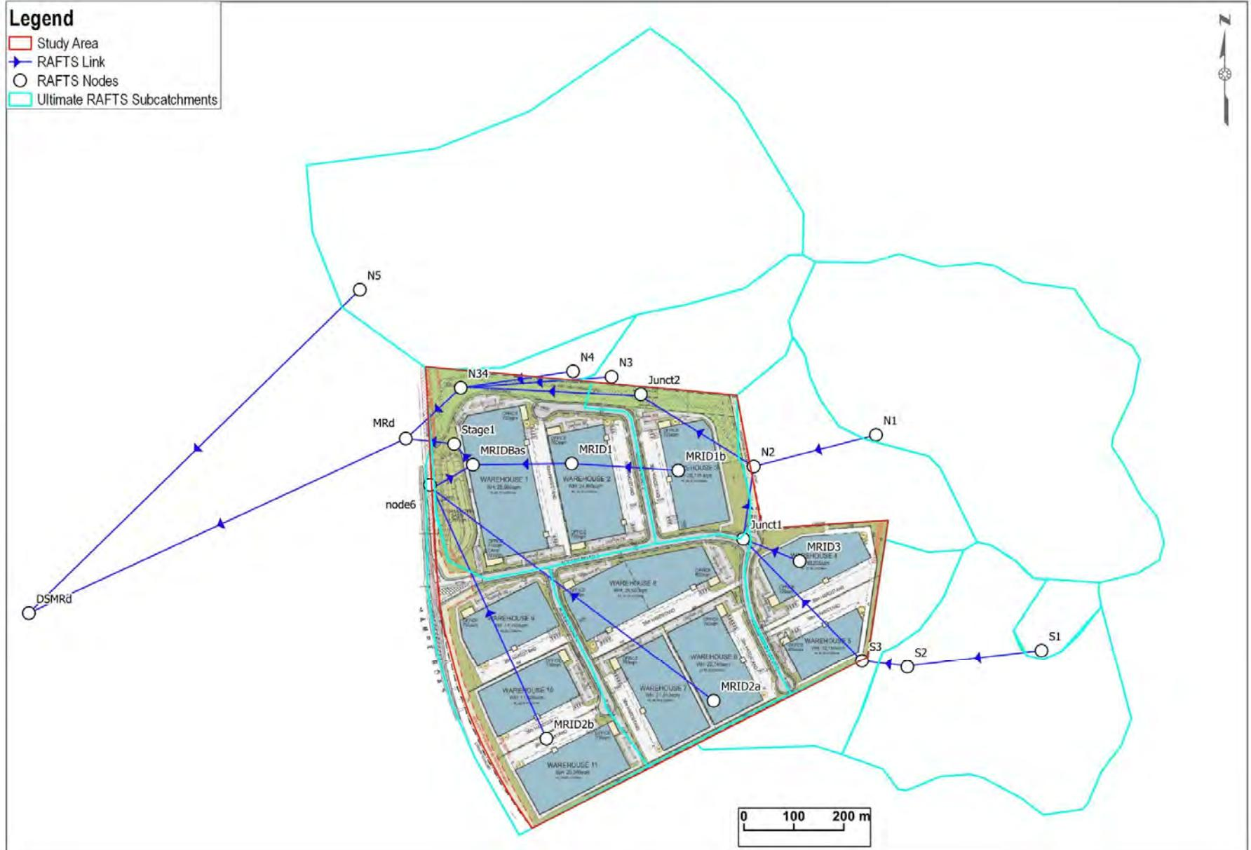
Figure 3 Local Subcatchment Boundaries in AIE XP-RAFTS model under Final Masterplan Conditions
