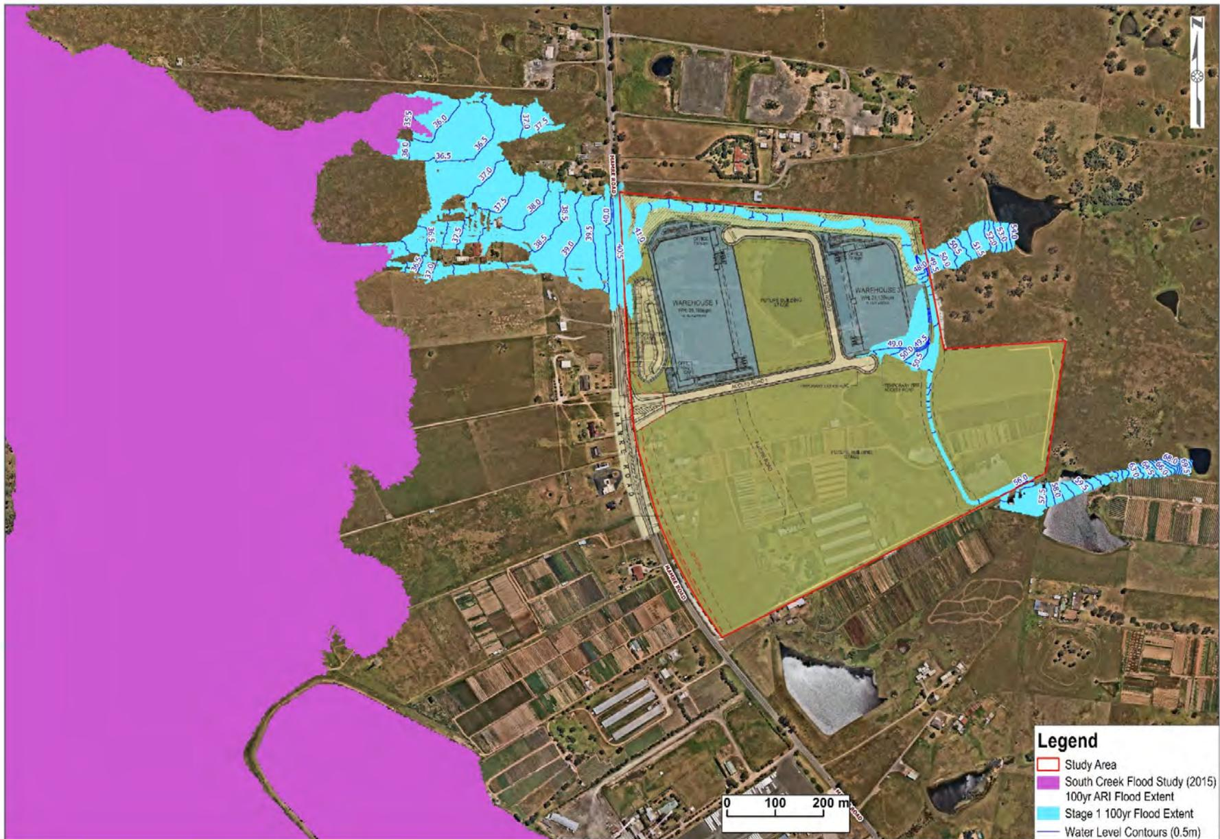
Figure 20 100 yr ARI Flood Extents and Flood Levels - Stage 1 Conditions
