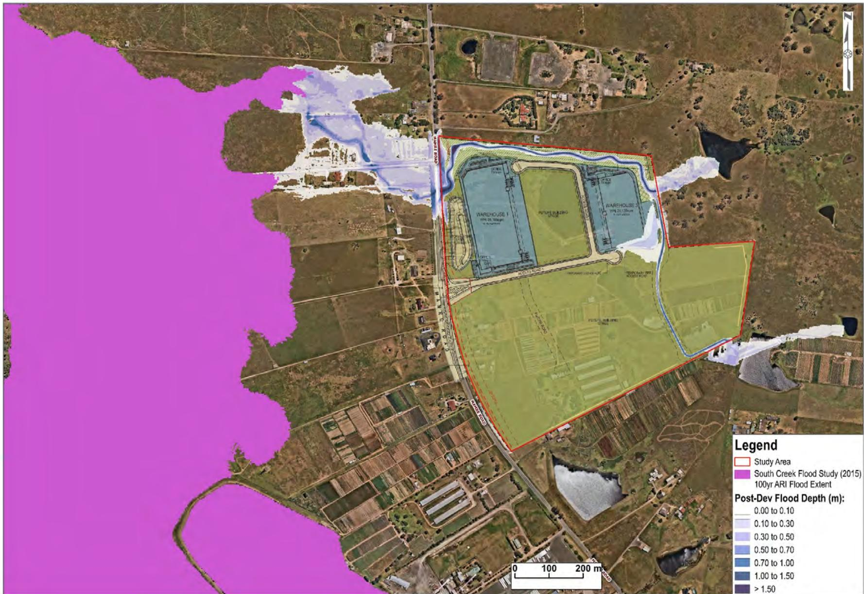
Figure 21 100 yr ARI Flood Depths - Stage 1 Conditions
