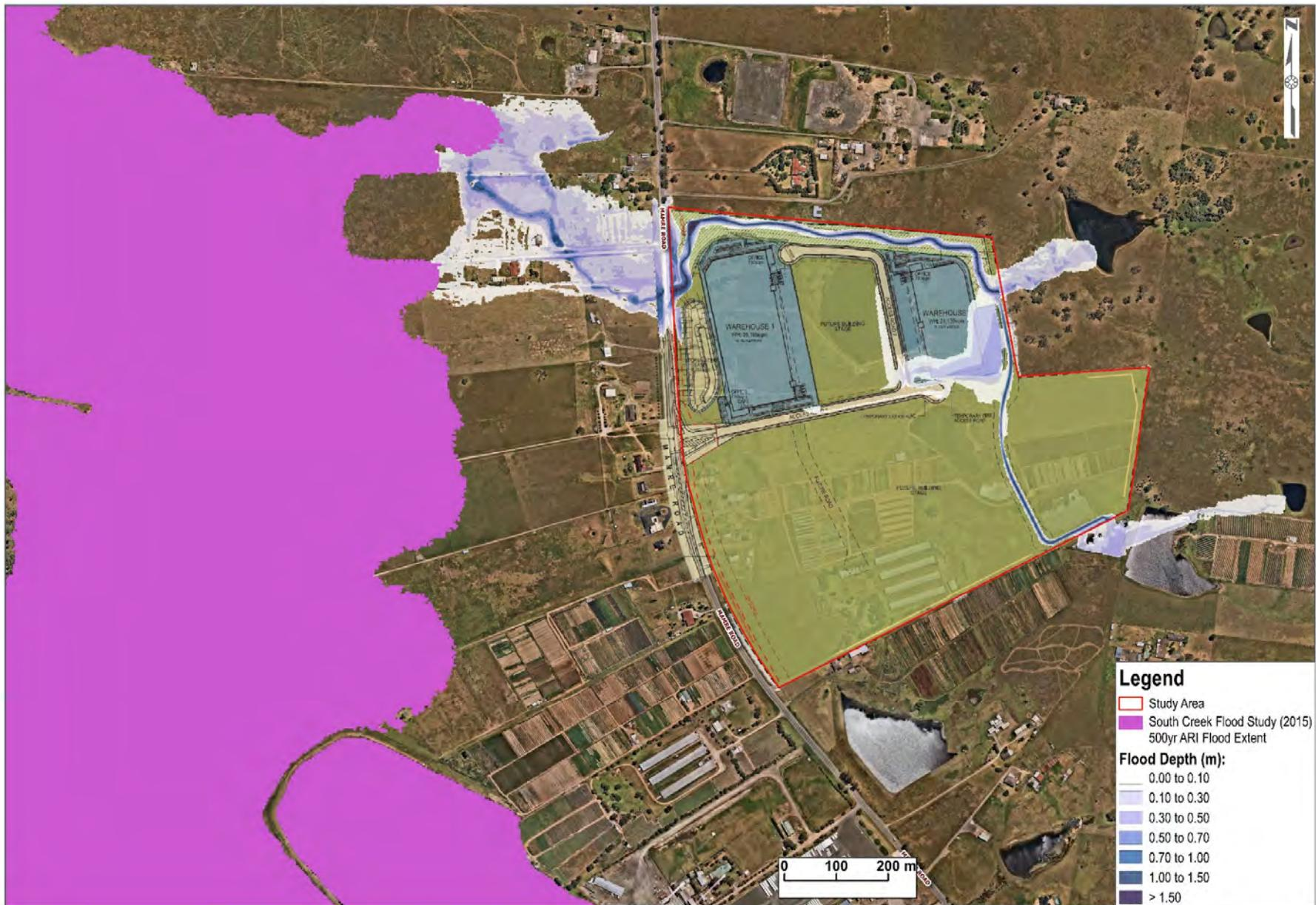
Figure 33 500 yr ARI Flood Depths - Stage 1 Conditions
