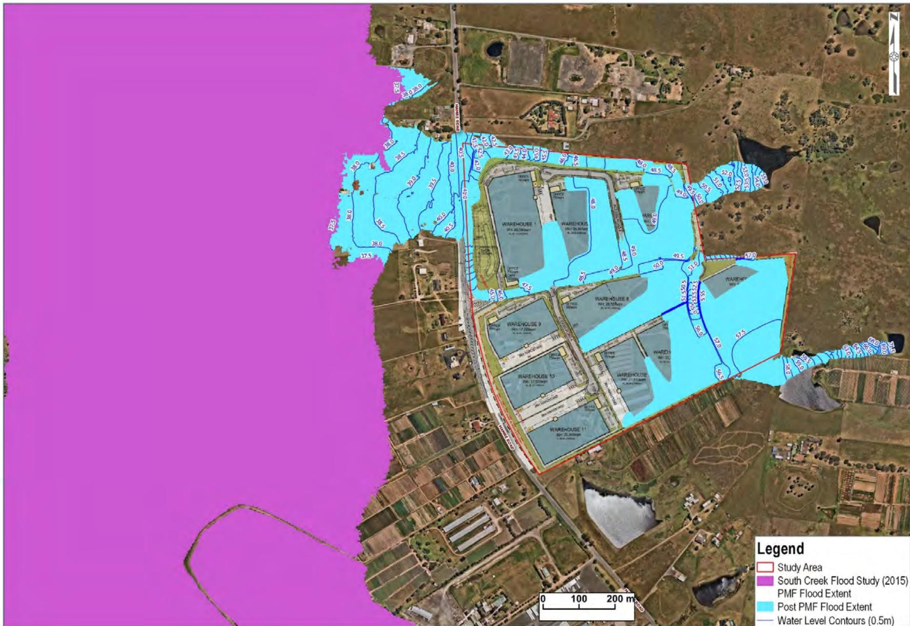
**Figure 74 PMF Flood Extents and Flood Levels - Final Masterplan Conditions**
