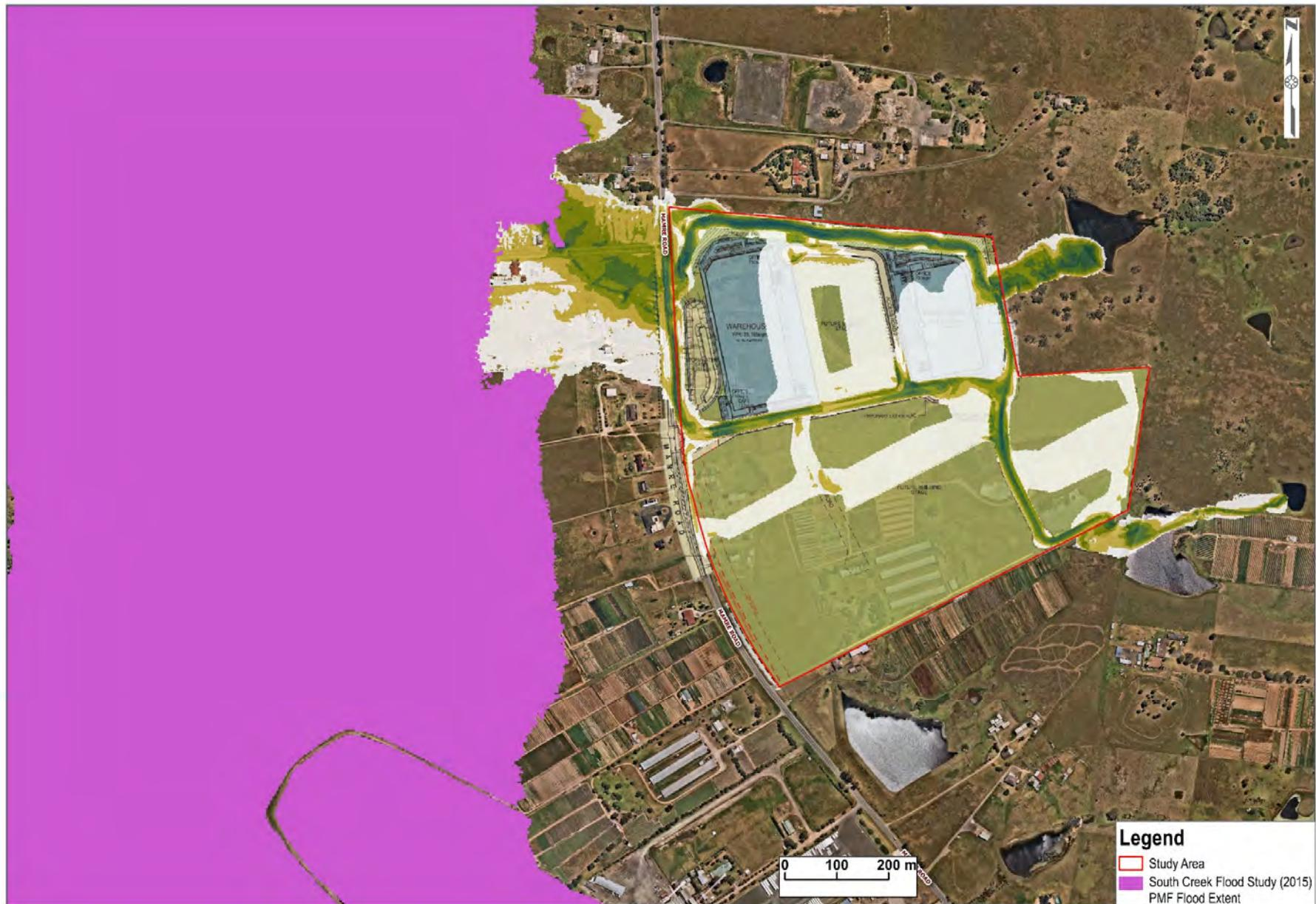
Figure 40 PMF Flood Velocities - Stage 1 Conditions
