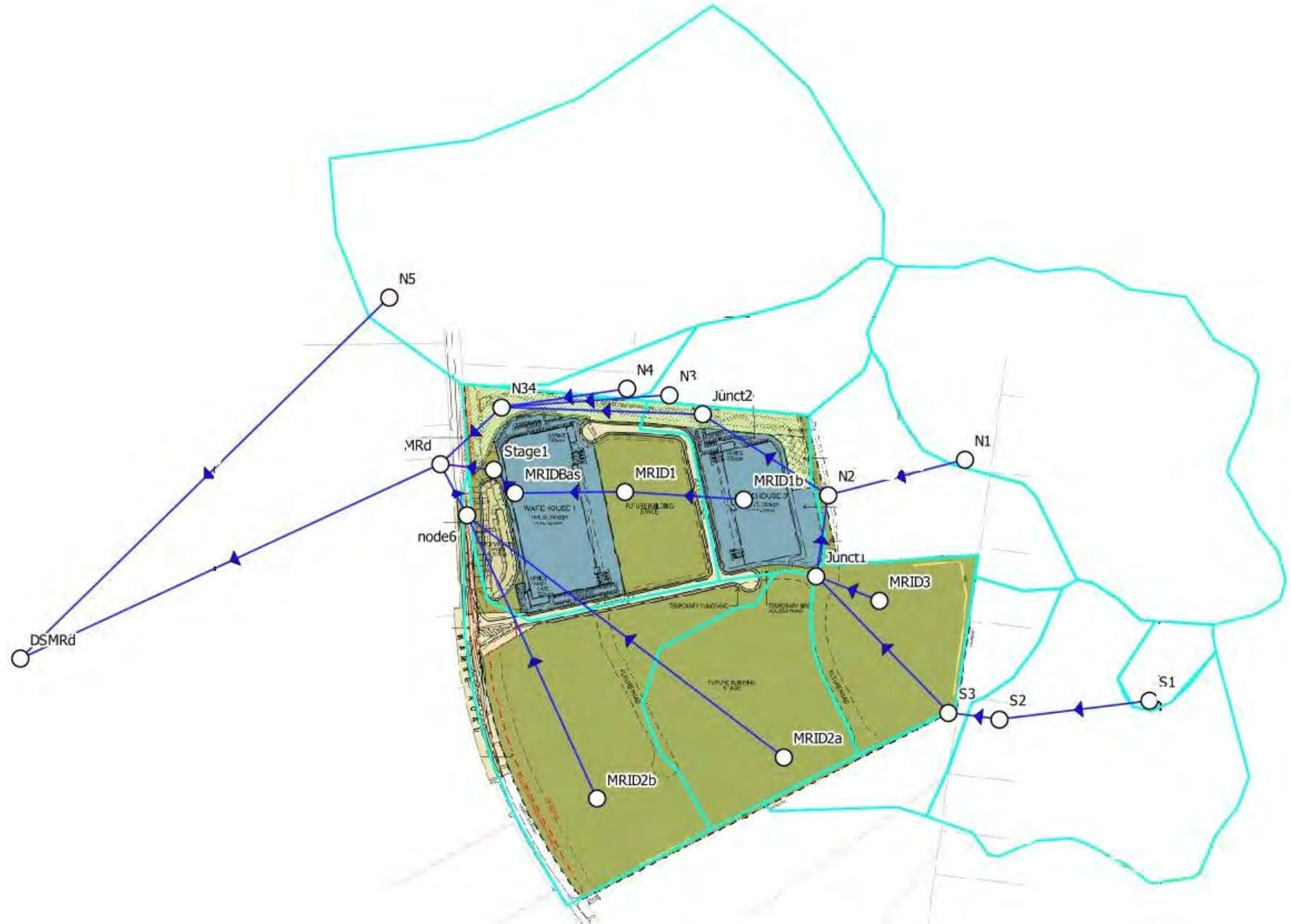
Figure 6 Local Subcatchment Boundaries in AIE XP-RAFTS model under Stage 1 Conditions
