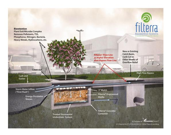
Stormwater flows through a specially designed filter media mixture contained in a landscaped concrete container. The mixture immobilizes pollutants which are then decomposed, volatilized and incorporated into the biomass of the Filterra® system's micro/macro fauna and flora. Stormwater runoff flows through the media and into an underdrain system at the bottom of the container, where the treated water is discharged. Higher flows bypass the Filterra® to a downstream inlet or outfall.
