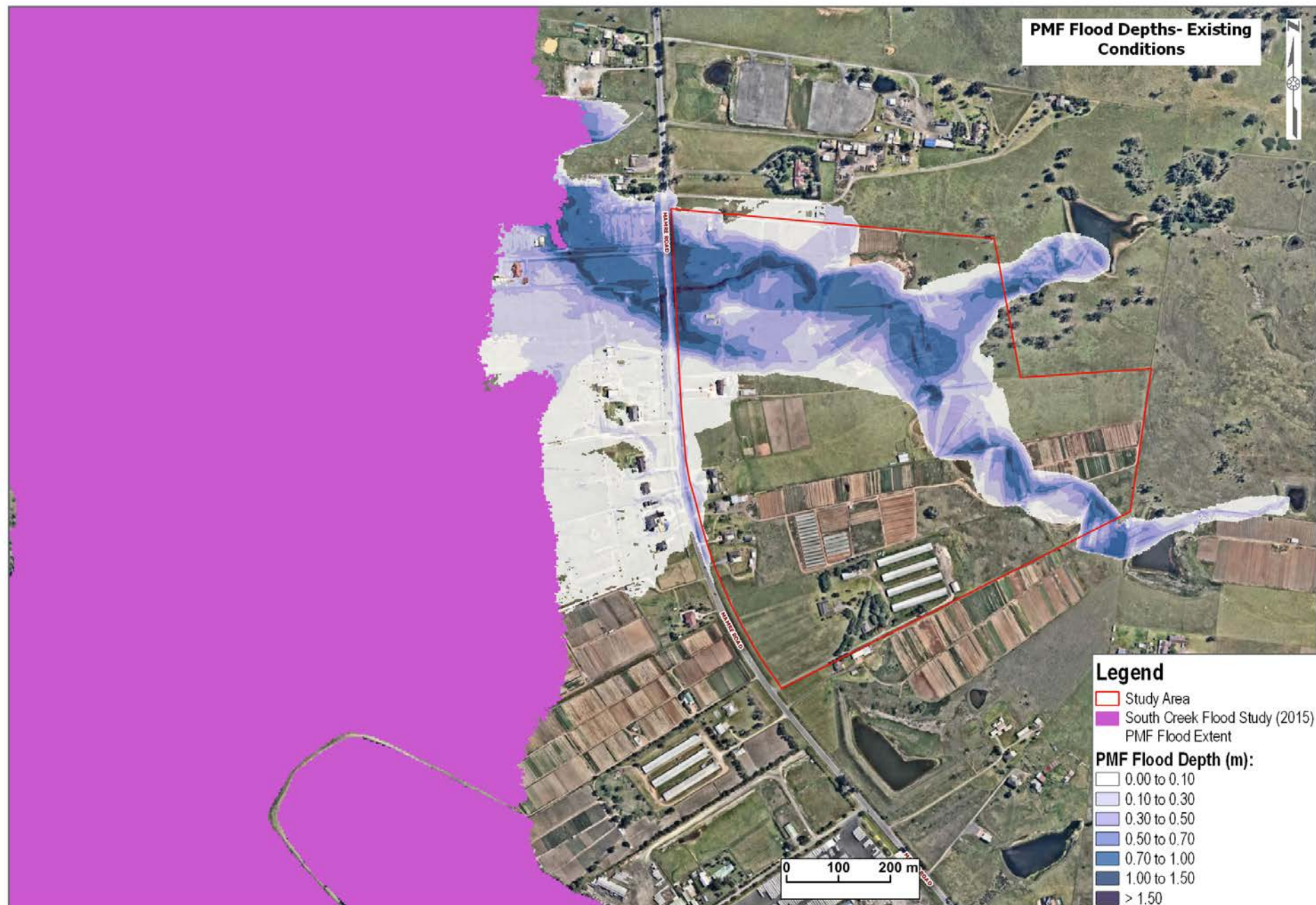
Figure 35 PMF Flood Depths - Benchmark Conditions
