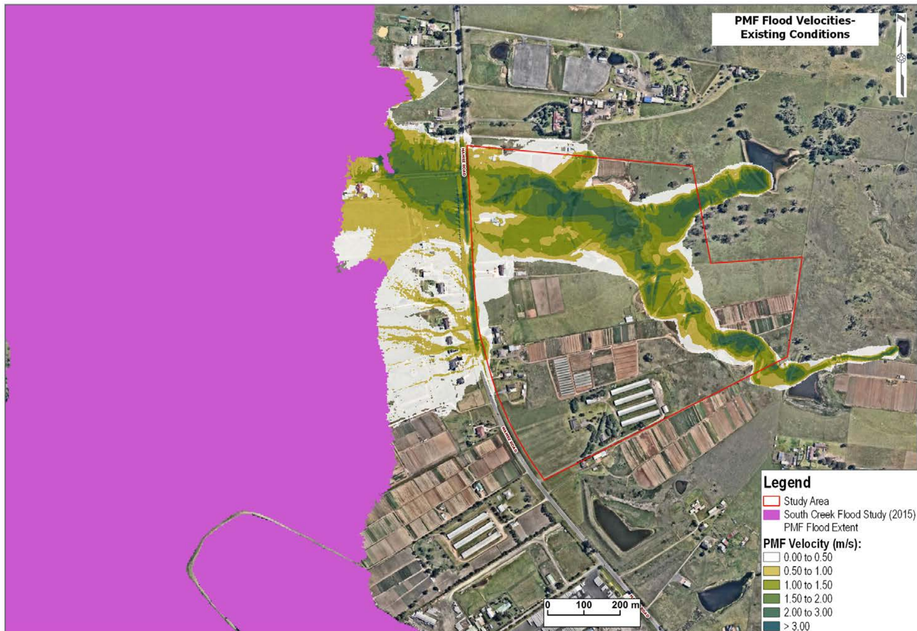
Figure 36 PMF Flood Velocities - Benchmark Conditions
