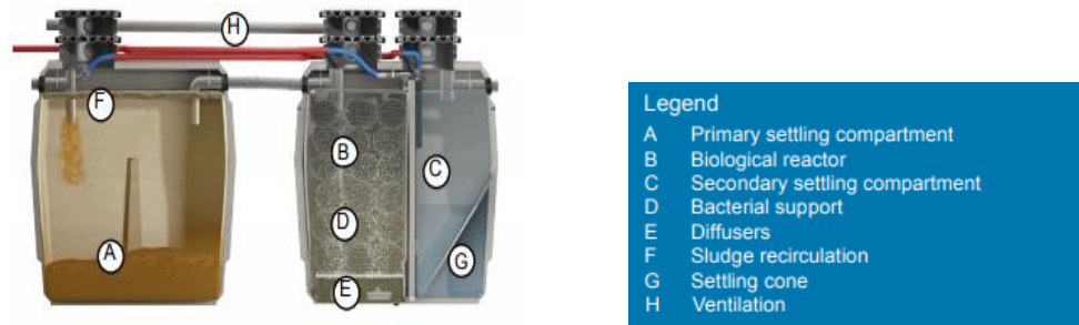
Figure 4 Oxy Fix Sewage (wastewater) Treatment Plant/Septic Tank Schematic
