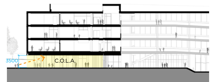
Secondary School: HUB Building undercroft
