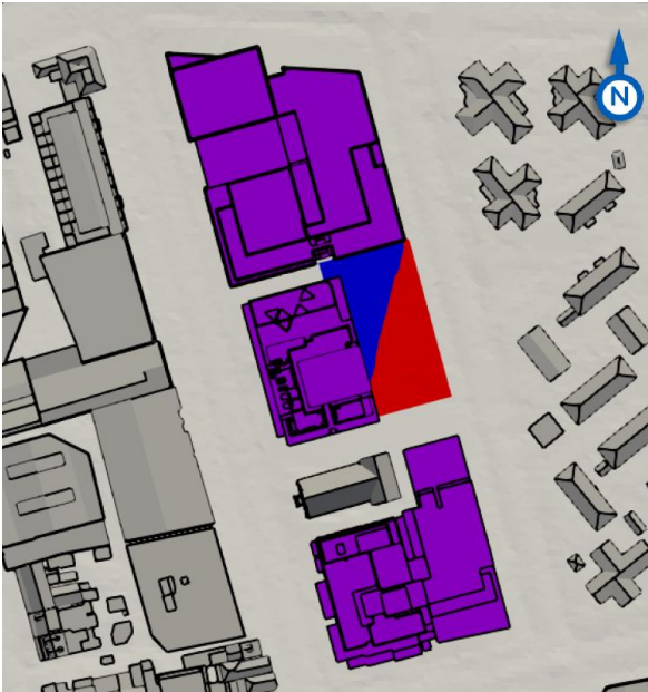
Figure 34 Area of Cope Street Plaza where direct solar access is available above 2 hours (red)
